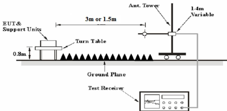
The radiated emission tests were performed in the 3 meters Semi-Anechoic Chamber, using the setup in accordance with the ANSI C63.4-2003. The specification used was the FCC 15.209 and FCC 15.247 limits.
