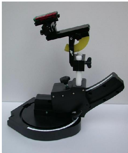
Device holder supplied by SPEAG
