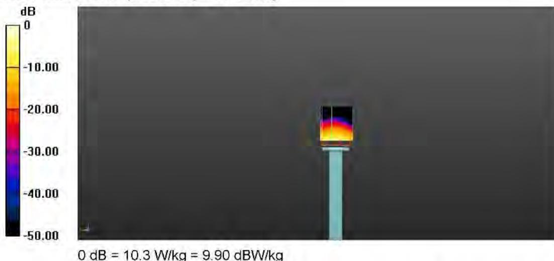
**Dipole validation measurement for Body Tissue/Pin= 100mW ,dist=10mm,f=5800 MHz /Zoom Scan (7x7x21)/Cube 0:**
