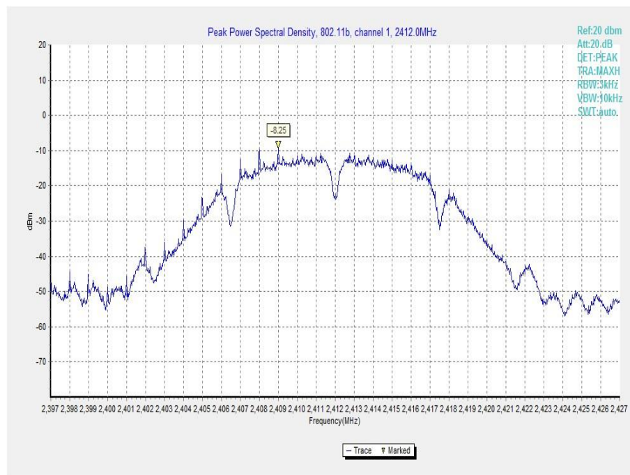
Fig.A.3.1 Power Spectral Density(802.11b,Ch1)
