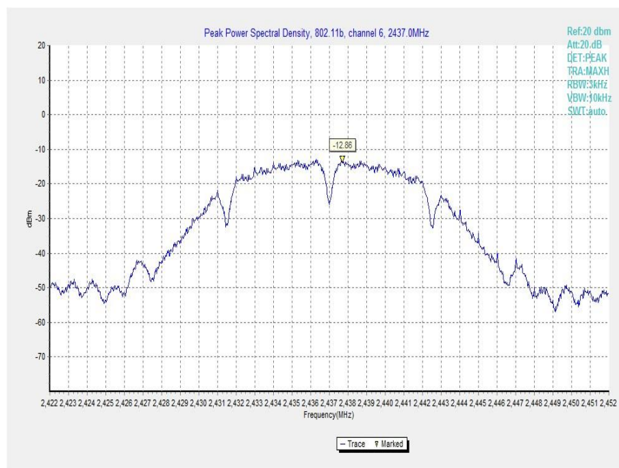
Fig.A.3.2 Power Spectral Density (802.11b, Ch 6)
