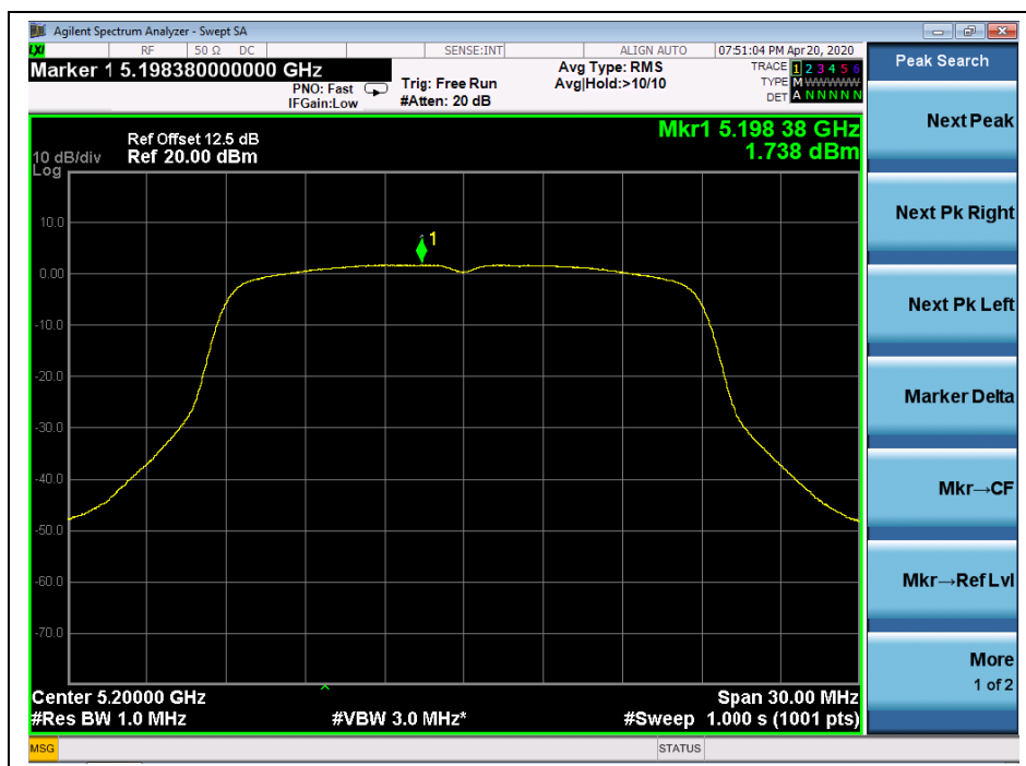
(Channel 44, 5220 MHz, 802.11ac (VHT20))
