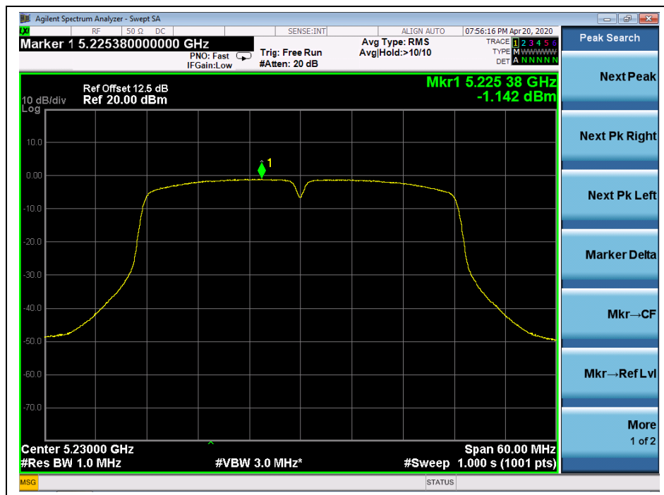
(Channel 46, 5230 MHz, 802.11ac (VHT40))
