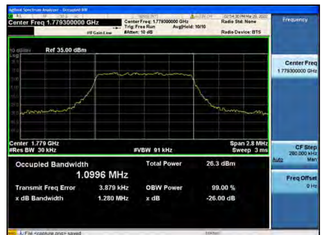
Band66 / 1.4MHz / High CH / 16QAM
