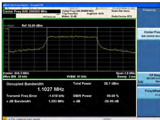
Band26Part22 / 1.4MHz / High CH / QPSK
