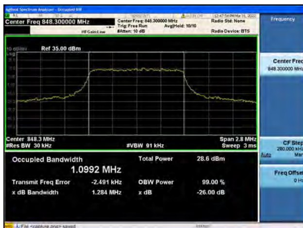
Band5 / 1.4MHz / High CH / QPSK
