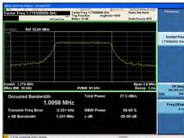
Band66 / 1.4MHz / High CH / QPSK
