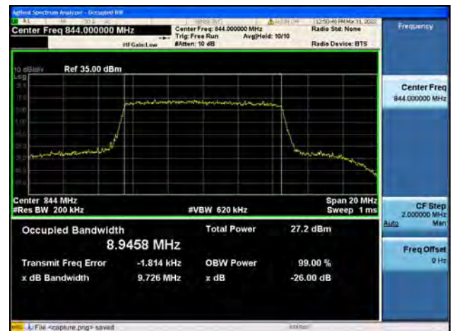
Band5 / 10MHz / High CH / 16QAM
