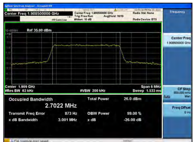
Band2 / 3MHz / High CH / 16QAM
