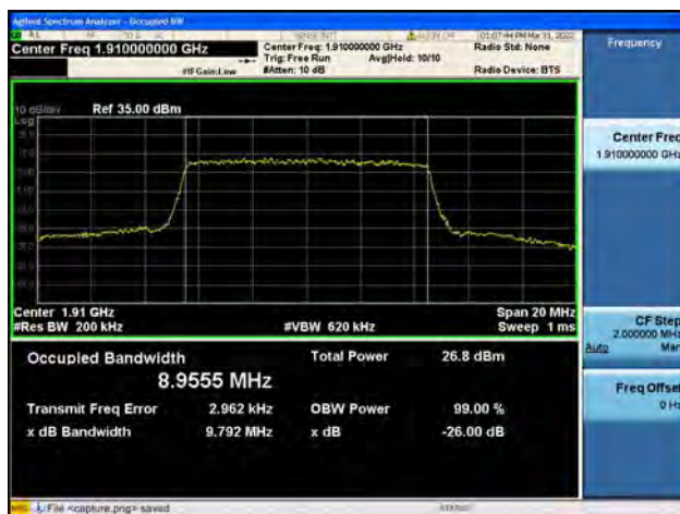
Band25 / 10MHz / High CH / QPSK
