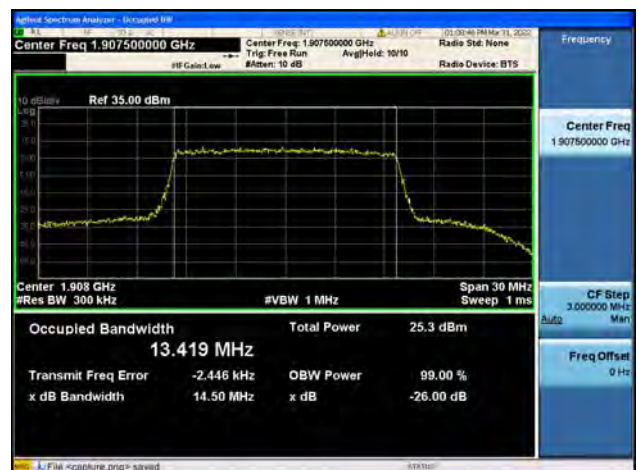
Band25 / 15MHz / High CH / 16QAM
