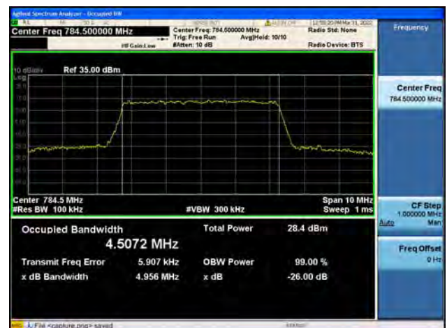
Band13 / 5MHz / High CH / 16QAM
