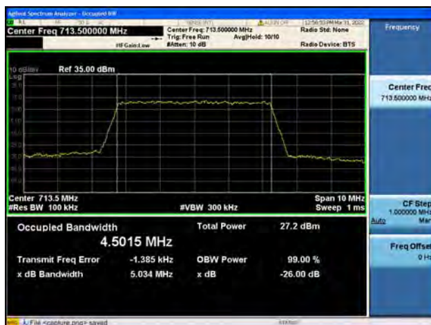
Band17 / 5MHz / High CH / QPSK
