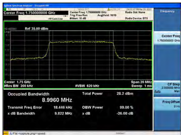
Band4 / 10MHz / High CH / QPSK
