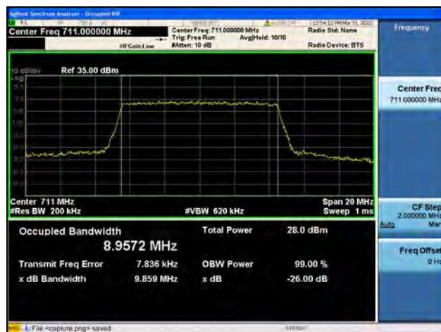
Band12 / 10MHz / High CH / QPSK
