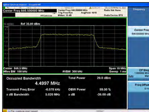
Band26Part22 / 5MHz / High CH / QPSK
