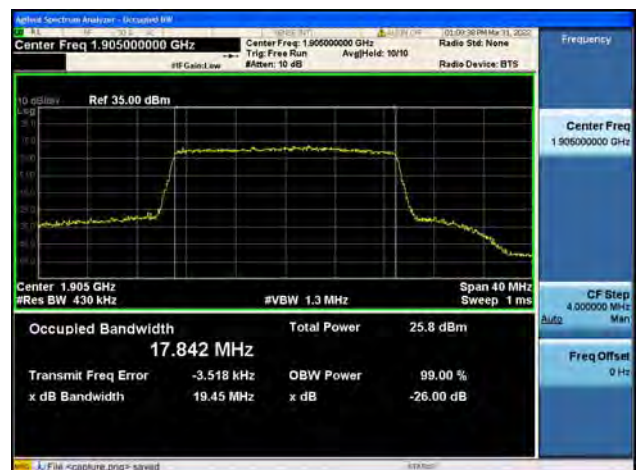
Band25 / 20MHz / High CH / 16QAM
