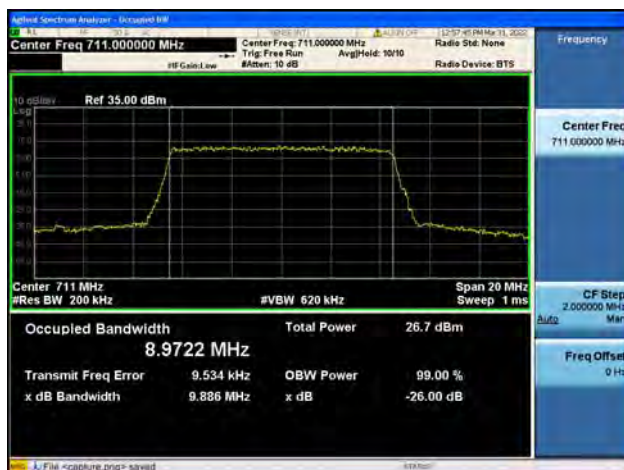
Band17 / 10MHz / High CH / QPSK
