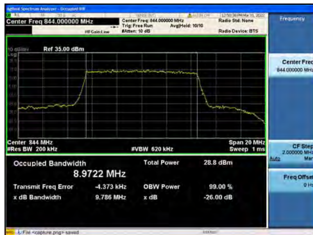
Band5 / 10MHz / High CH / QPSK
