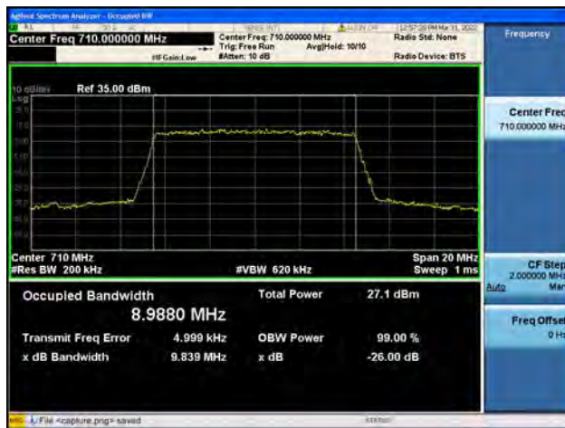
Band17 / 10MHz / High CH / QPSK
