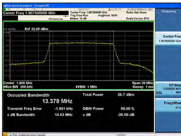
Band25 / 15MHz / High CH / QPSK
