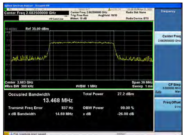
Band41 / 15MHz / High CH / 16QAM
