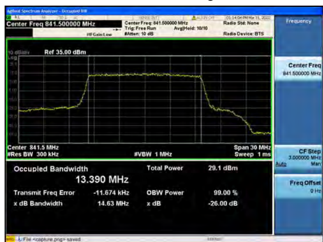
Band26Part22 / 15MHz / High CH / QPSK
