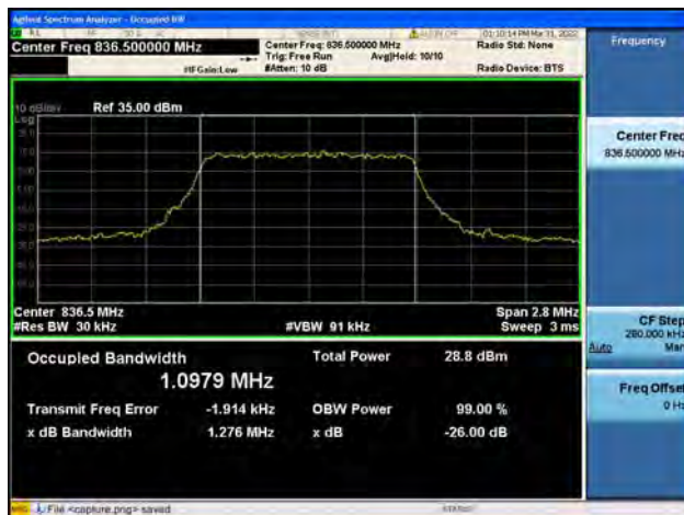
Band26Part22 / 1.4MHz / High CH / QPSK
