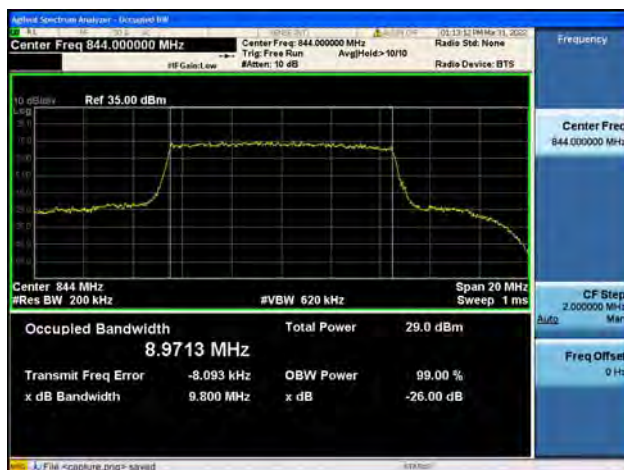
Band26Part22 / 10MHz / High CH / QPSK
