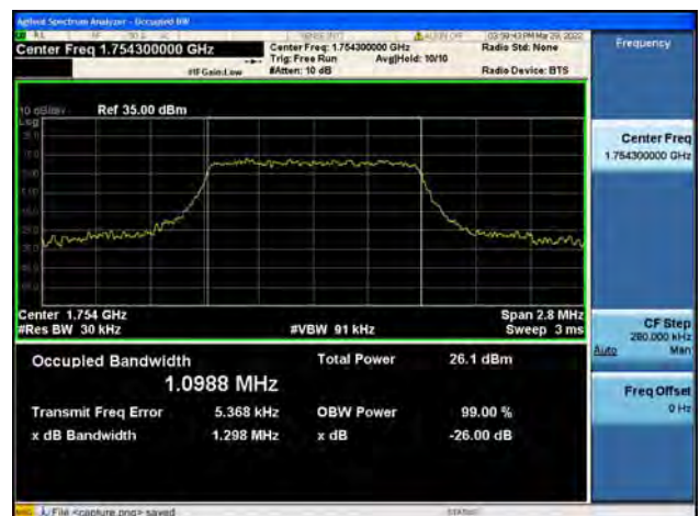
Band4 / 1.4MHz / High CH / 16QAM
