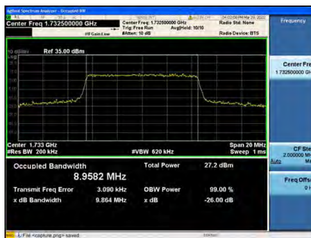
Band4 / 10MHz / High CH / 16QAM
