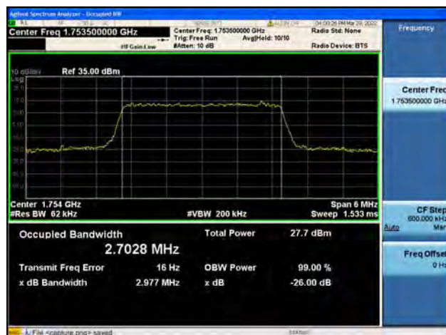
Band4 / 3MHz / High CH / QPSK
