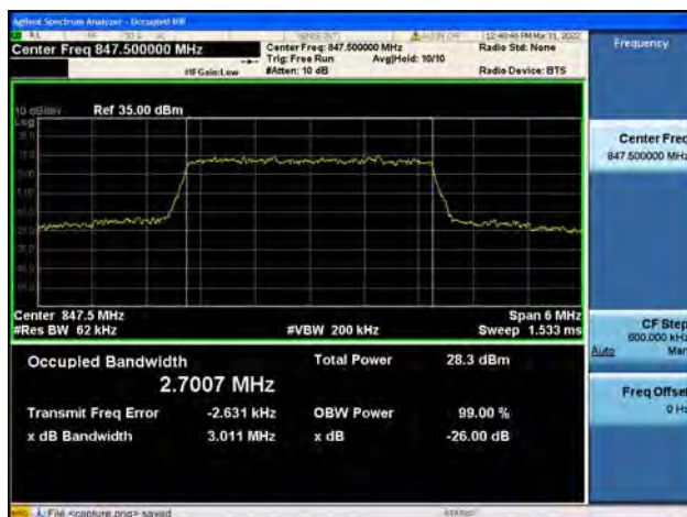
Band5 / 3MHz / High CH / QPSK
