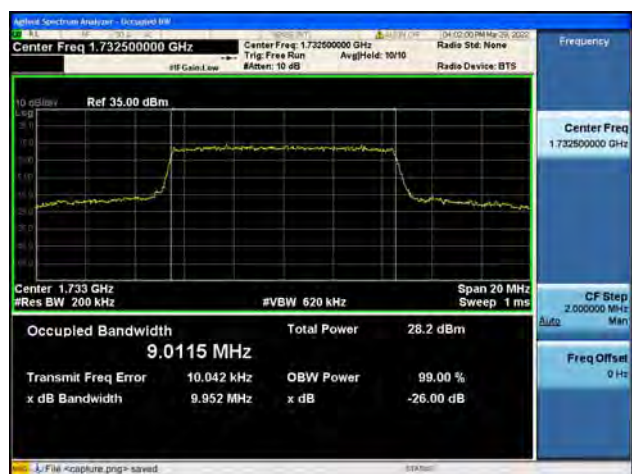
Band4 / 10MHz / High CH / QPSK
