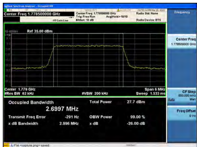
Band66 / 3MHz / High CH / QPSK
