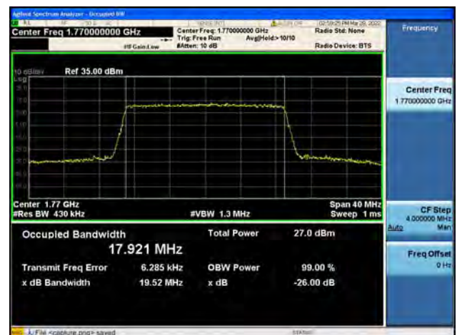
Band66 / 20MHz / High CH / 16QAM
