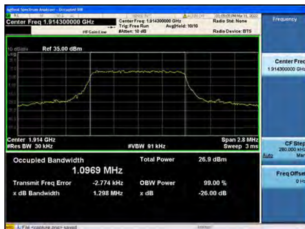
Band25 / 1.4MHz / High CH / QPSK
