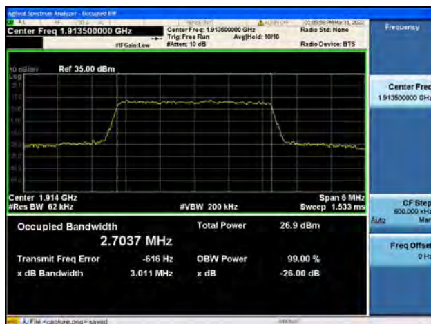
Band25 / 3MHz / High CH / QPSK
