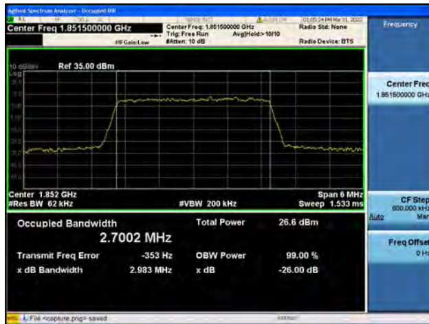
Band25 / 3MHz / Mid CH / QPSK
