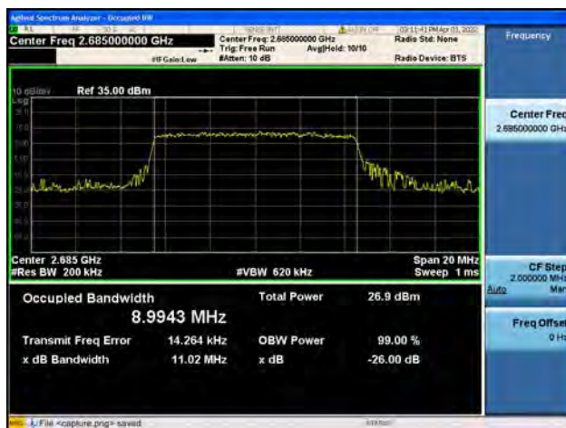
Band41 / 10MHz / High CH / QPSK
