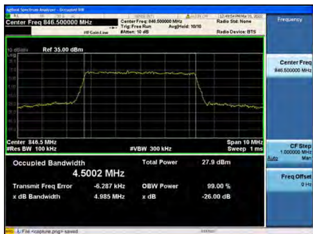
Band5 / 5MHz / High CH / 16QAM
