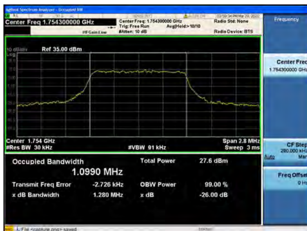
Band4 / 1.4MHz / High CH / QPSK
