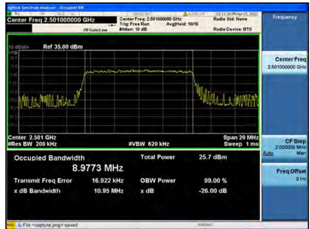
Band41 / 10MHz / Mid CH / 16QAM
