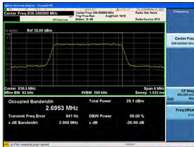
Band26Part22 / 3MHz / High CH / QPSK
