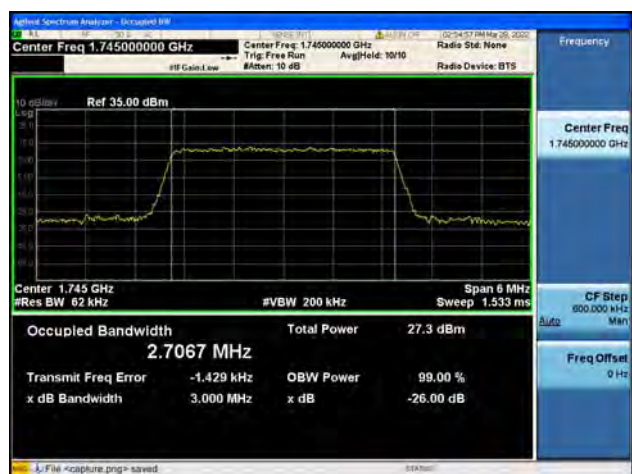
Band66 / 3MHz / High CH / QPSK
