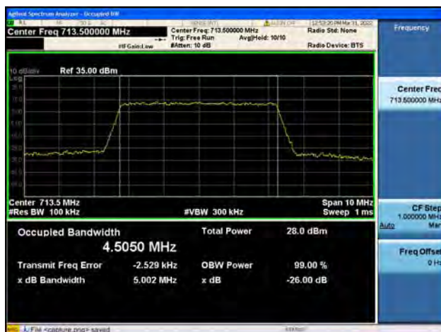
Band12 / 5MHz / High CH / QPSK
