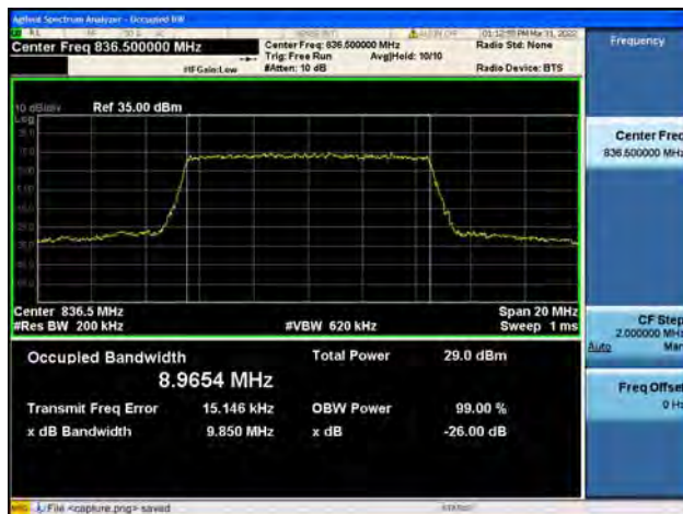
Band26Part22 / 10MHz / High CH / QPSK
