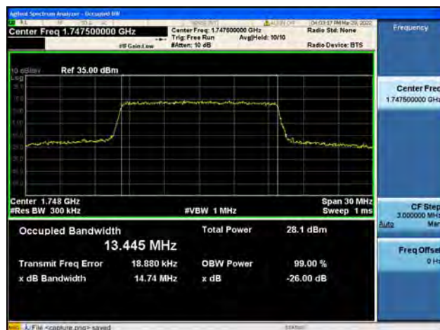
Band4 / 15MHz / High CH / QPSK
