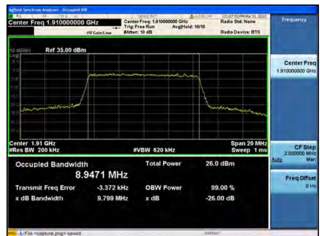
Band25 / 10MHz / High CH / 16QAM
