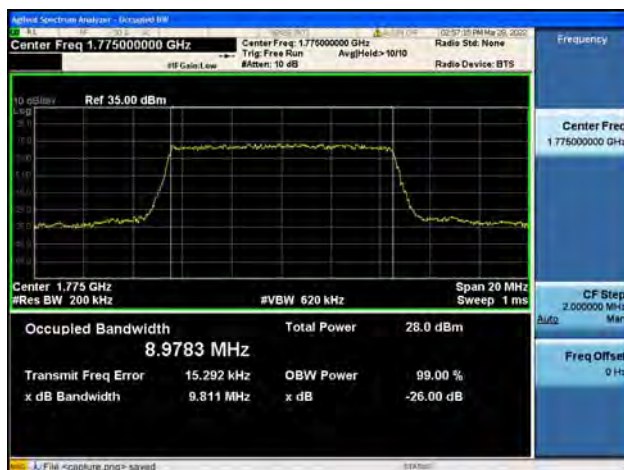
Band66 / 10MHz / High CH / QPSK
