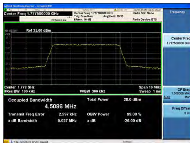
Band66 / 5MHz / High CH / QPSK
