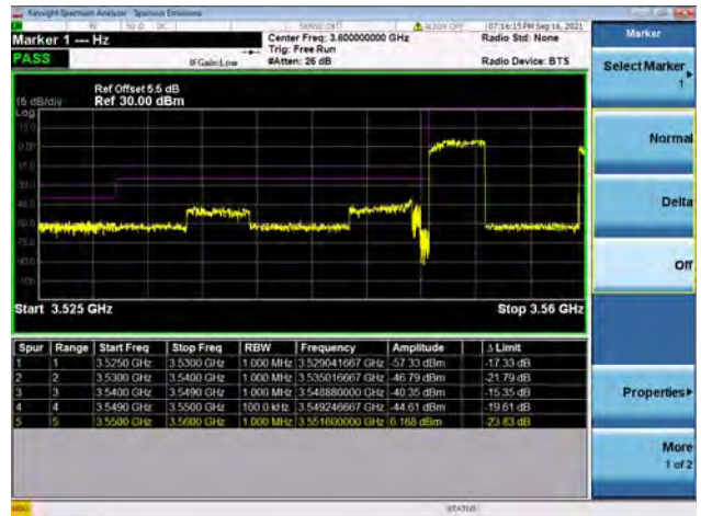
Band48 / 10MHz / High CH / QPSK / FULL RB
