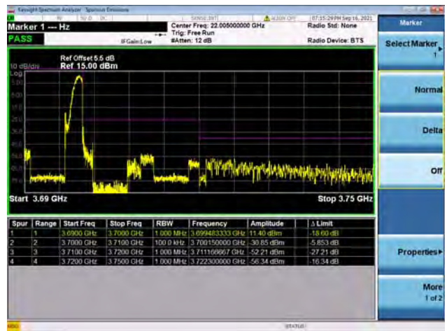
Band48 / 10MHz / High CH / QPSK / FULL RB
