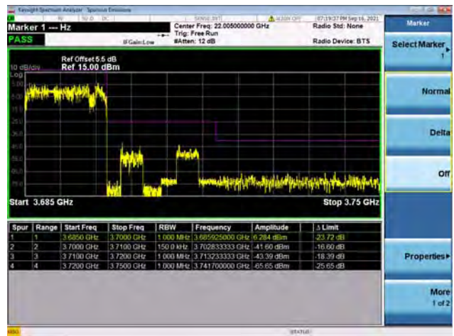
Band48 / 15MHz / High CH / QPSK / FULL RB
