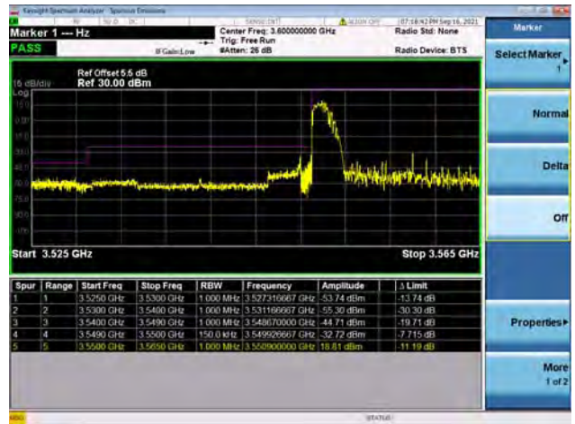
Band48 / 15MHz / High CH / QPSK / FULL RB
