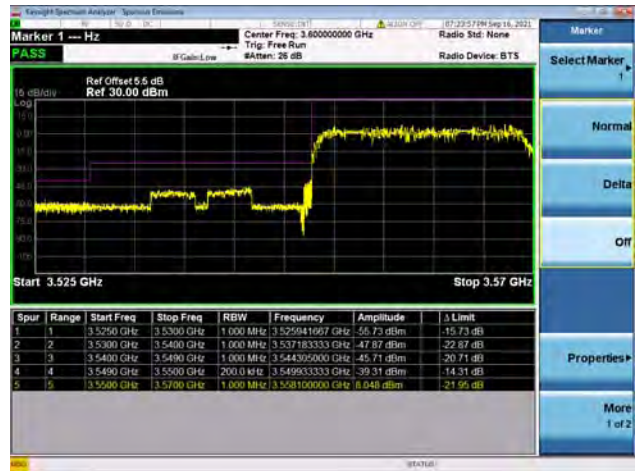
Band48 / 20MHz / High CH / QPSK / FULL RB
