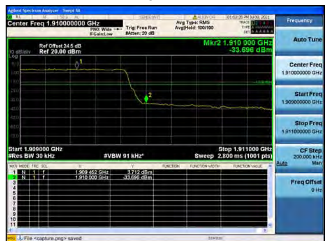
Band2 / 3MHz / Low CH / QPSK / FULL RB
