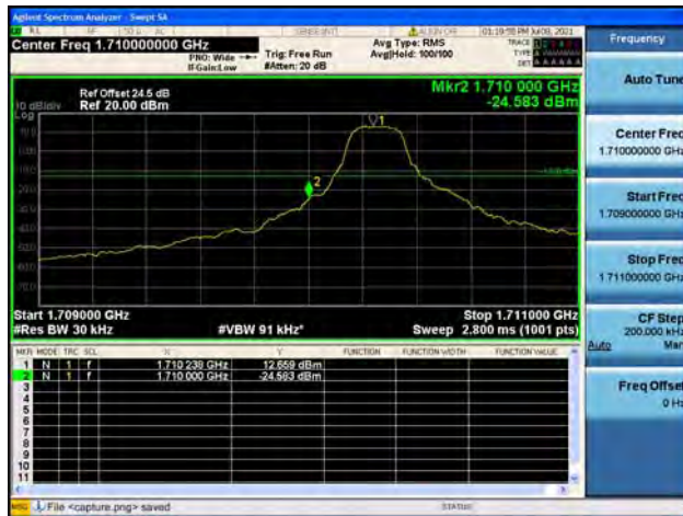
Band4 / 1.4MHz / High CH / QPSK / 1 RB
