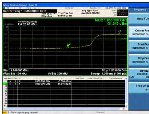
Band2 / 10MHz / High CH / QPSK / FULL RB
