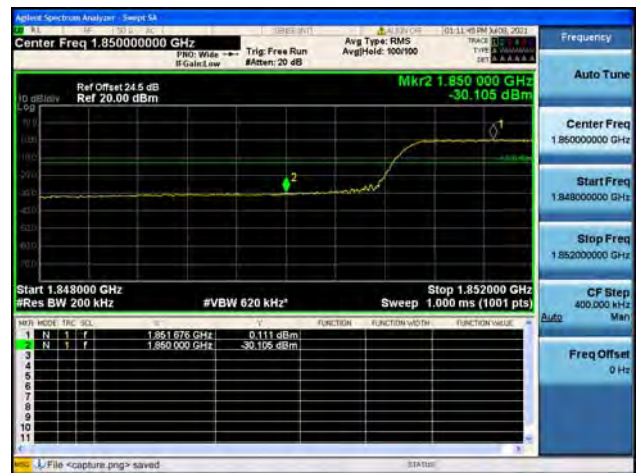
Band2 / 20MHz / High CH / QPSK / FULL RB
