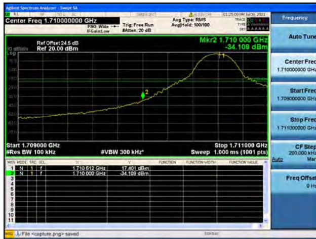
Band4 / 10MHz / High CH / QPSK / 1 RB
