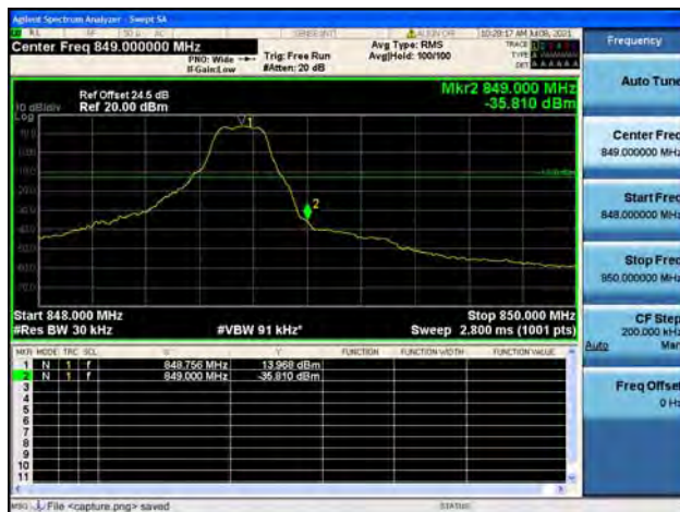
Band5 / 3MHz / Low CH / QPSK / 1 RB
