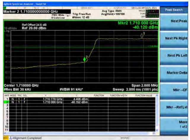
Band66 / 1.4MHz / High CH / QPSK / FULL RB
