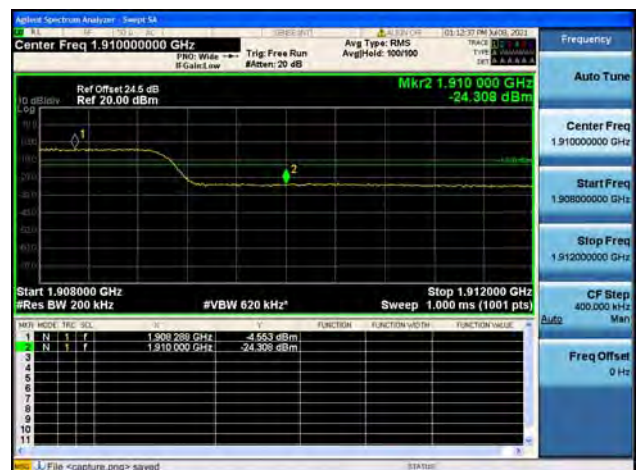
Band2 / 20MHz / High CH / QPSK / FULL RB
