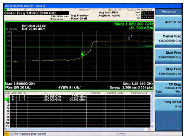
Band2 / 3MHz / Low CH / QPSK / FULL RB
