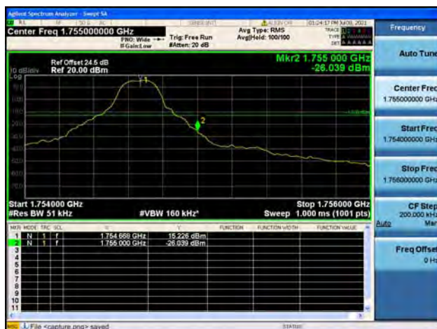
Band4 / 5MHz / High CH / QPSK / 1 RB
