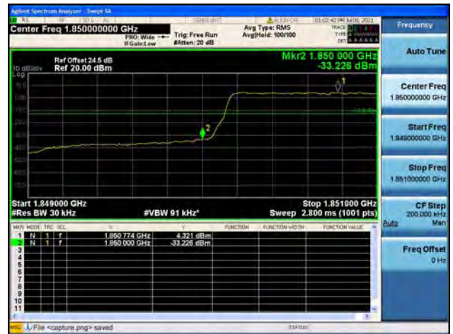
Band2 / 1.4MHz / High CH / QPSK / FULL RB
