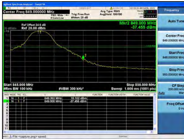
Band12 / 1.4MHz / Low CH / QPSK / 1 RB
