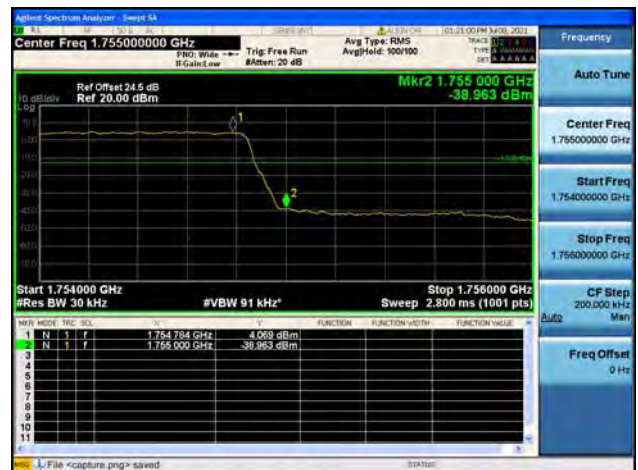
Band4 / 3MHz / Low CH / QPSK / FULL RB
