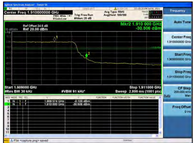
Band2 / 5MHz / Low CH / QPSK / FULL RB
