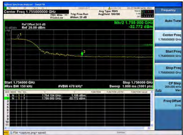
Band4 / 20MHz / Low CH / QPSK / FULL RB
