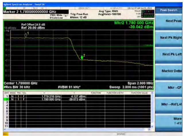
Band66 / 1.4MHz / High CH / QPSK / FULL RB
