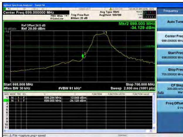
Band12 / 1.4MHz / Low CH / QPSK / 1 RB
