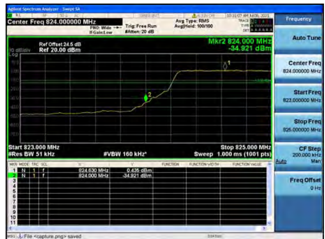
Band5 / 5MHz / High CH / QPSK / FULL RB
