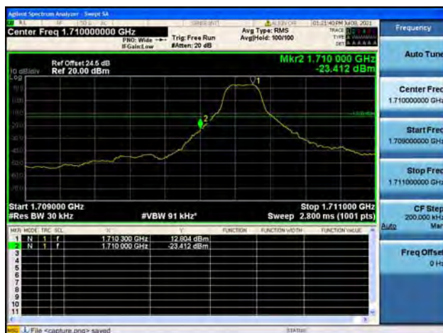
Band4 / 3MHz / Low CH / QPSK / 1 RB
