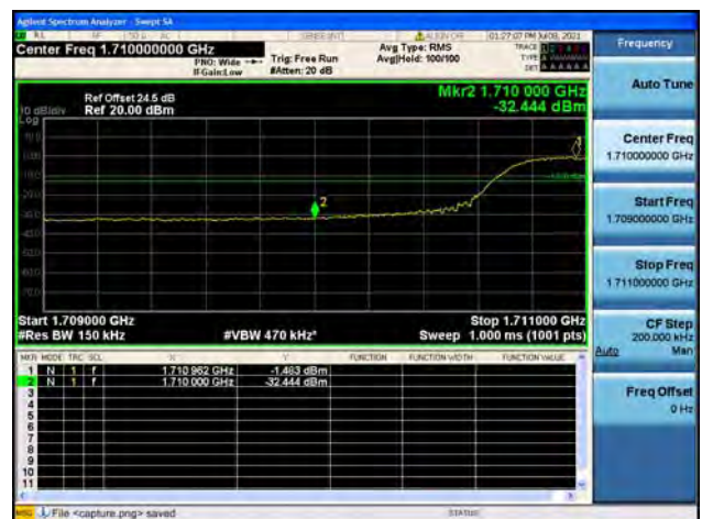
Band4 / 15MHz / Low CH / QPSK / FULL RB
