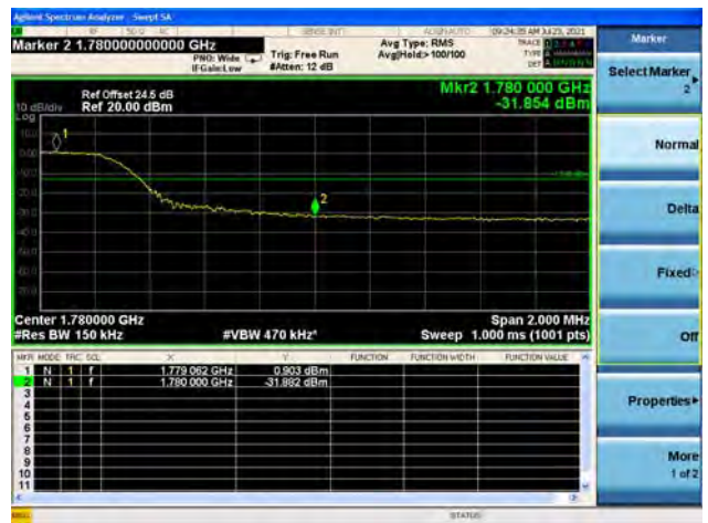
Band66 / 15MHz / High CH / QPSK / FULL RB
