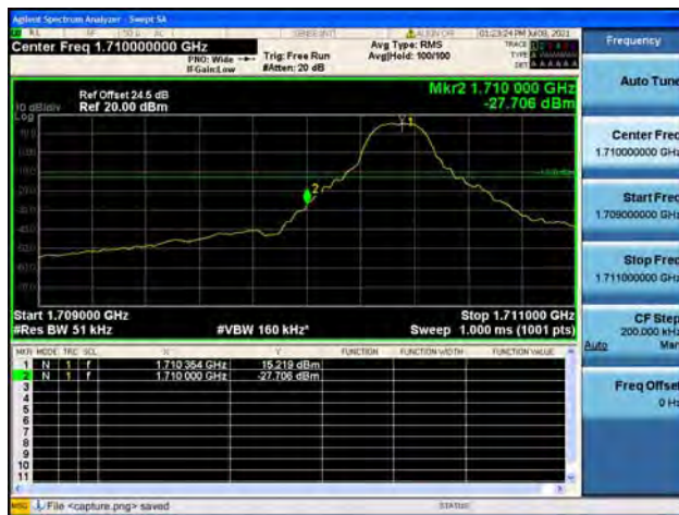
Band4 / 5MHz / High CH / QPSK / 1 RB
