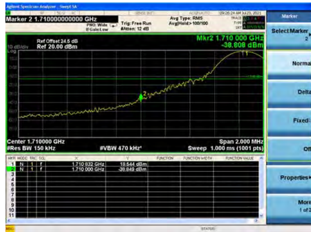
Band66 / 15MHz / High CH / QPSK / 1 RB
