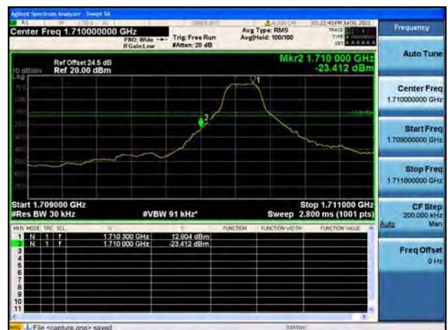
Band4 / 3MHz / Low CH / QPSK / FULL RB
