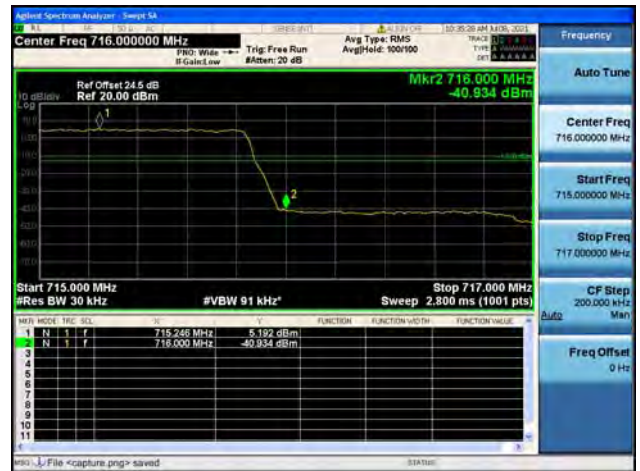
Band12 / 3MHz / Low CH / QPSK / FULL RB
