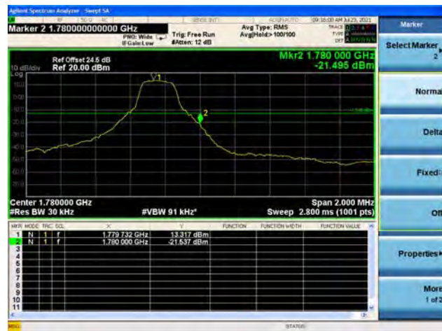
Band66 / 3MHz / High CH / QPSK / 1 RB
