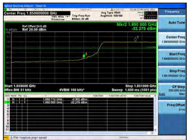
Band2 / 5MHz / High CH / QPSK / FULL RB
