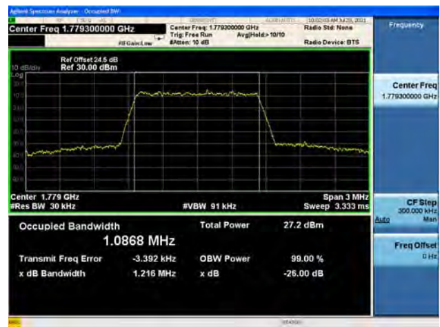
Band66 / 3MHz / Low CH / QPSK
