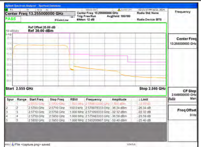
B7 / 15MHz / High CH / QPSK / FULL RB
