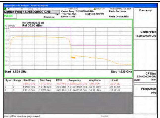
B2 / 15MHz / High CH / QPSK / FULL RB
