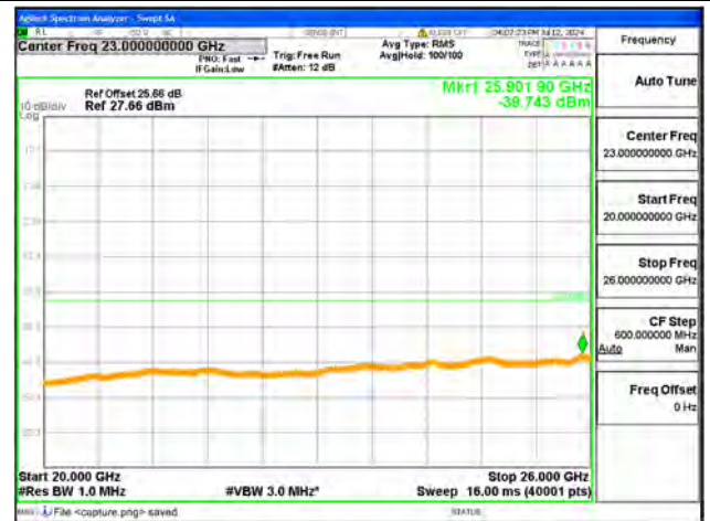
B7-20G-26G / 15MHz / Mid CH / QPSK
