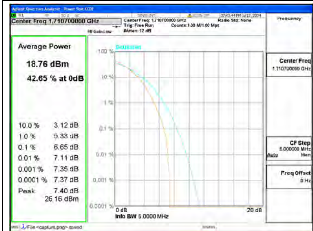
B4 / 1.4MHz / Low CH / 64QAM
