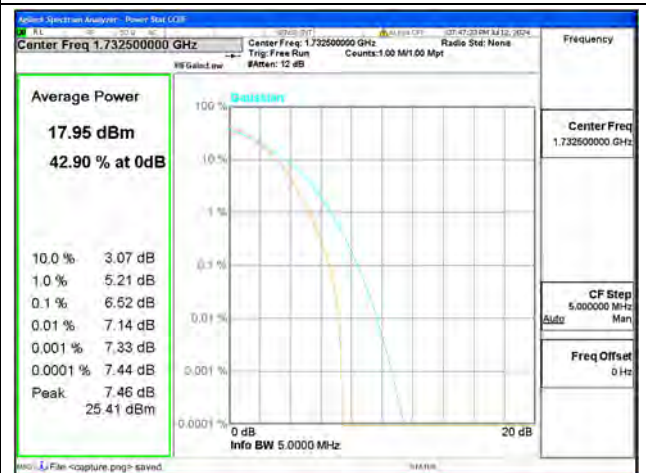
B4 / 5MHz / Mid CH / 64QAM
