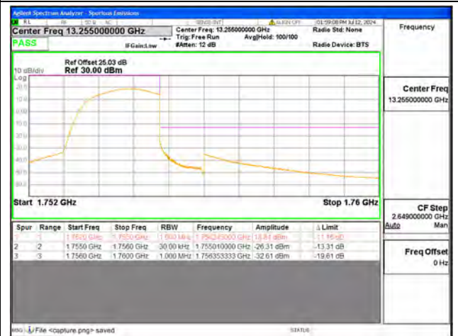
B4 / 1.4MHz / High CH / QPSK / FULL RB
