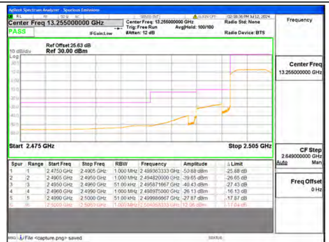
B7 / 5MHz / Low CH / QPSK / FULL RB
