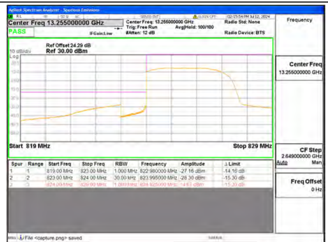
B5 / 3MHz / Low CH / QPSK / FULL RB
