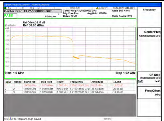
B2 / 10MHz / High CH / QPSK / FULL RB
