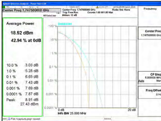
B4 / 15MHz / High CH / 64QAM
