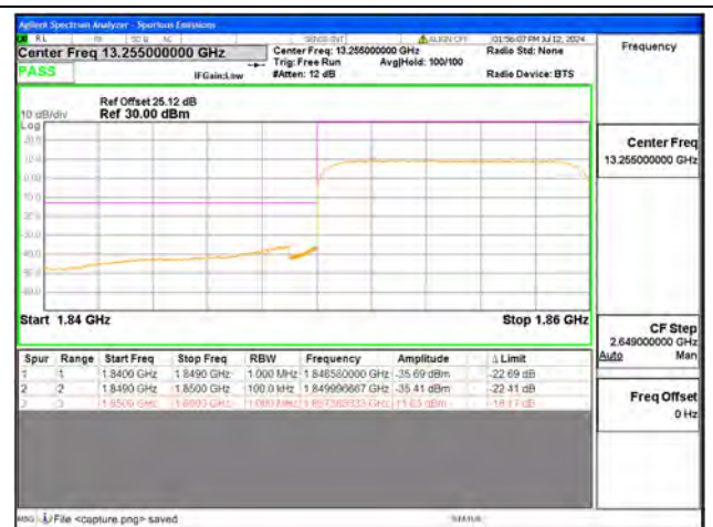
B2 / 10MHz / Low CH / QPSK / FULL RB
