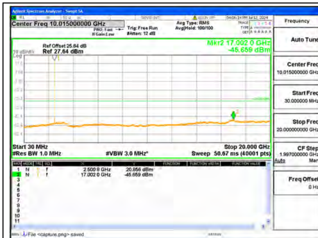
B7-30M-20G / 15MHz / Low CH / QPSK
