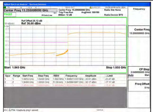
B2 / 5MHz / Low CH / QPSK / FULL RB
