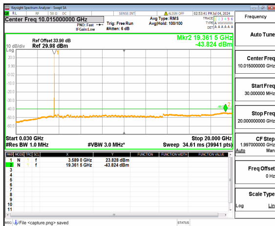
n48 (30MHz-20GHz) 40M DFT-s-OFDM BPSK Inner_1RB_Right Low
