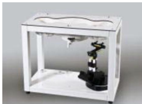
Fig. 6.8 Photo of SAM Phantom
