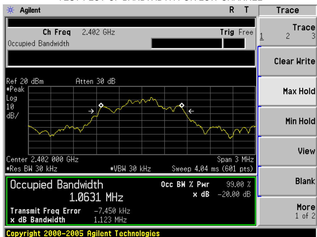
TEST PLOT OF BANDWIDTH FOR LOW CHANNEL
