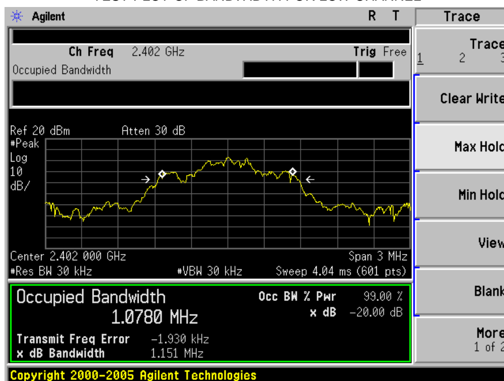
TEST PLOT OF BANDWIDTH FOR LOW CHANNEL
