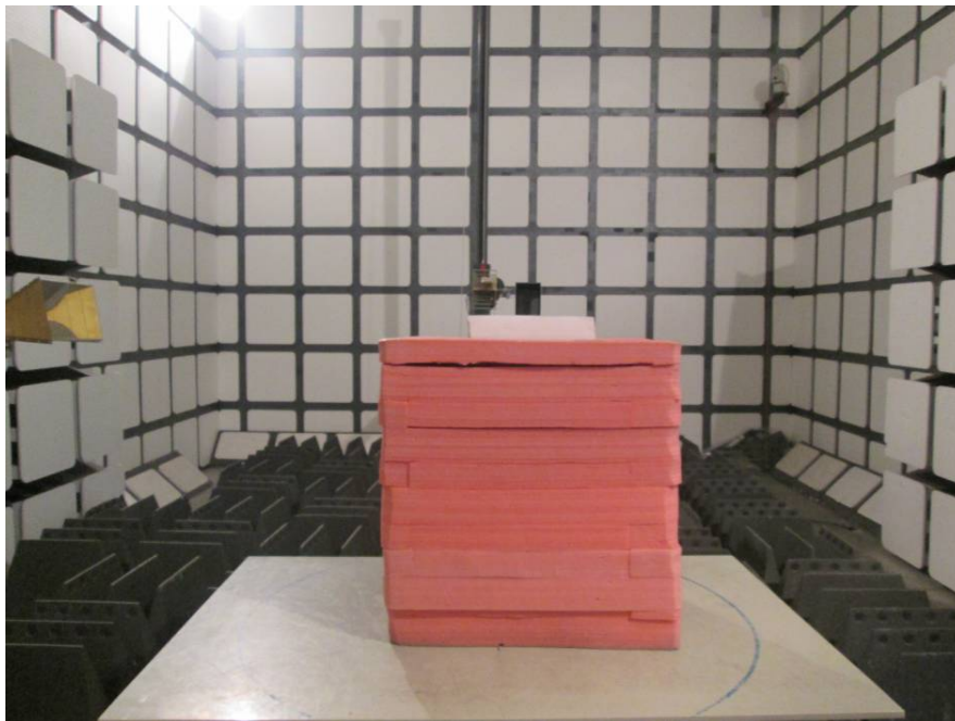
Radiated Emissions Test View (Above 1 GHz)
