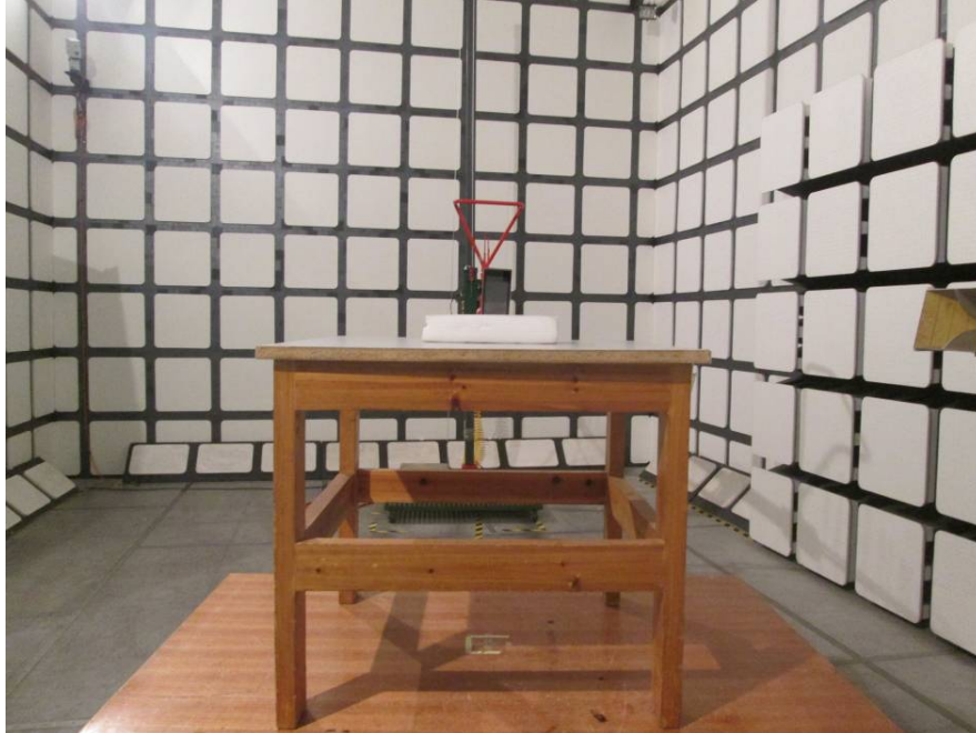
Radiated Emissions Test View (Below 1 GHz)
