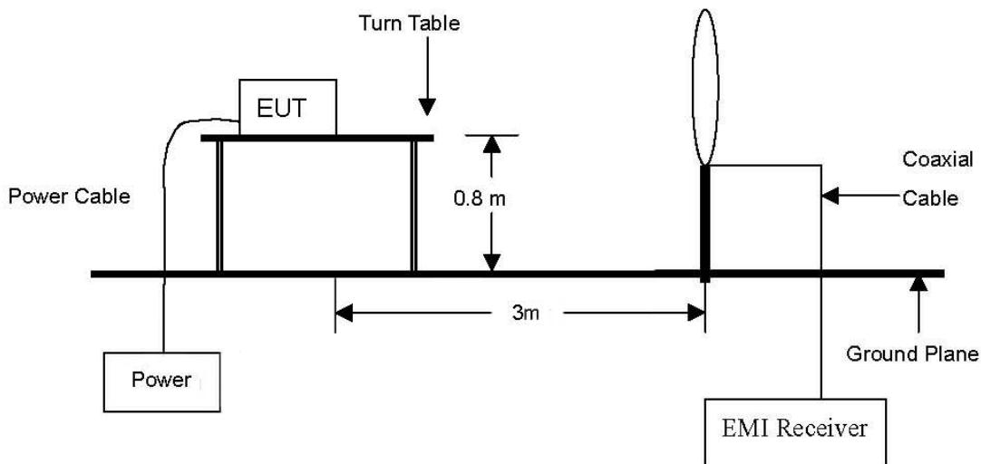
The diagram below shows the test setup that is utilized to make the measurements for emission from 30 MHz to 135.6 MHz Emissions.
