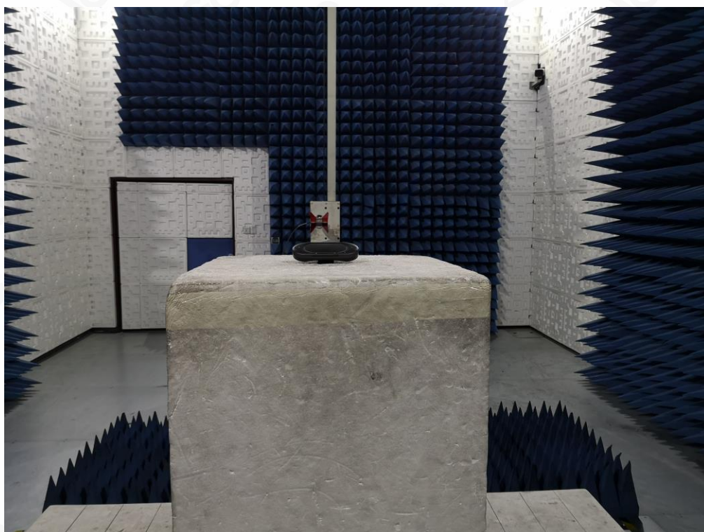
RADIATED EMISSION TEST SETUP ABOVE 1GHZ
