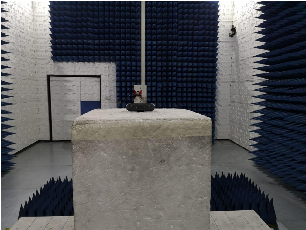
RADIATED EMISSION TEST SETUP ABOVE 1GHZ
