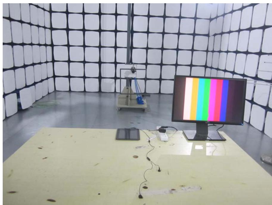
**Radiation Emission Test Setup (Below 1GHz)**
