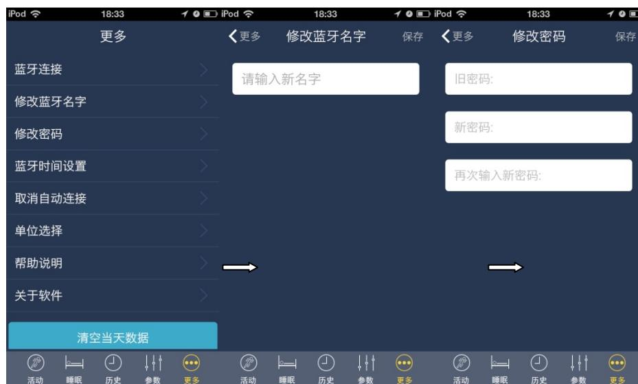
(9) **Time setting of Bluetooth and Automatic connection:** Close the automatic connection within the “More” interface, it saves the power of device. About the time setting, if the “Auto shut down” was closed, we can close Bluetooth manually; if it was open, the Bluetooth can be shut down auto, and the shut down time can be set from 1-120 minutes.
