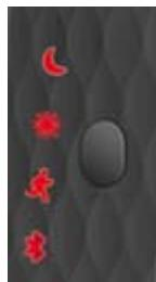
7.1 If the wristband is less than 5% power, fourled indicator lightsflash red; if less than 2% of power:fourred indicator lights are lighting up.
