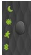
8.1 Put the inner core into the USB charging base, connect to PC USB Port, then four led lights flash green for 3 times after the existing status of led light flashes one time. It shows it is charging normally.
