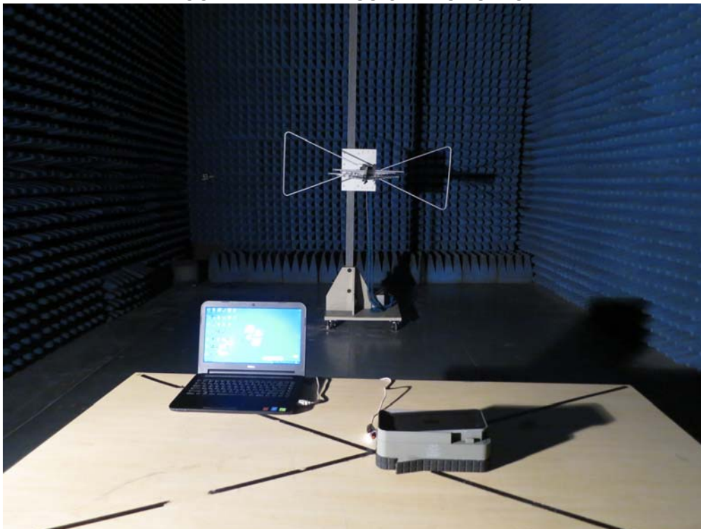
FCC RADIATED EMISSION TEST SETUP
