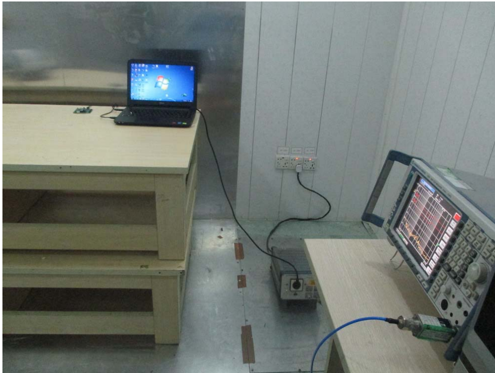
FCC RADIATED EMISSION TEST SETUP
