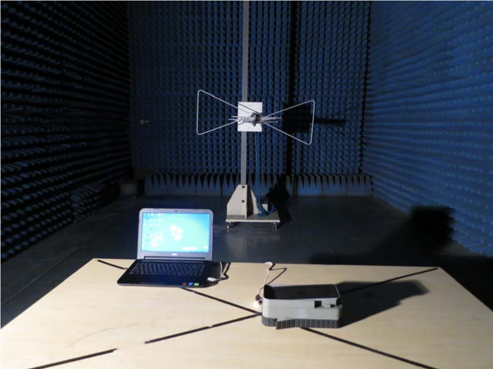
FCC RADIATED EMISSION TEST SETUP
