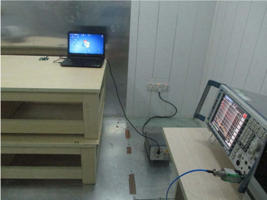
FCC RADIATED EMISSION TEST SETUP
