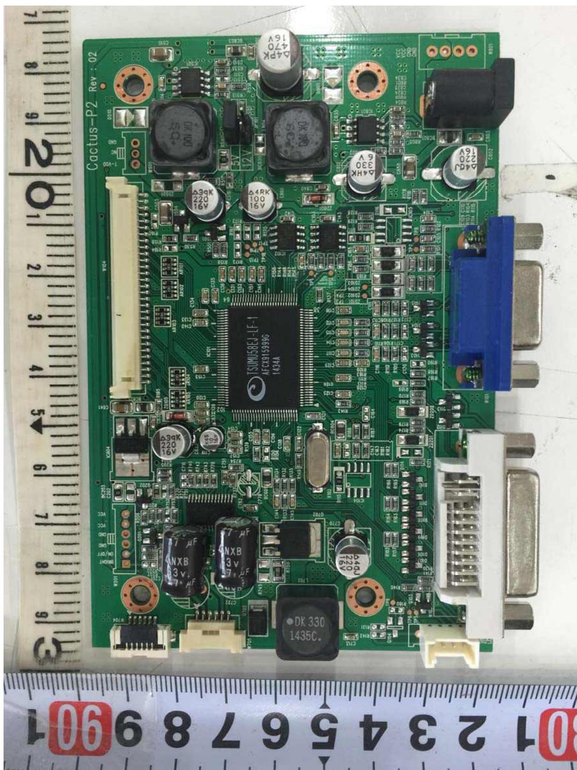
View of Main PCB of Monitor 1(Bottom)
