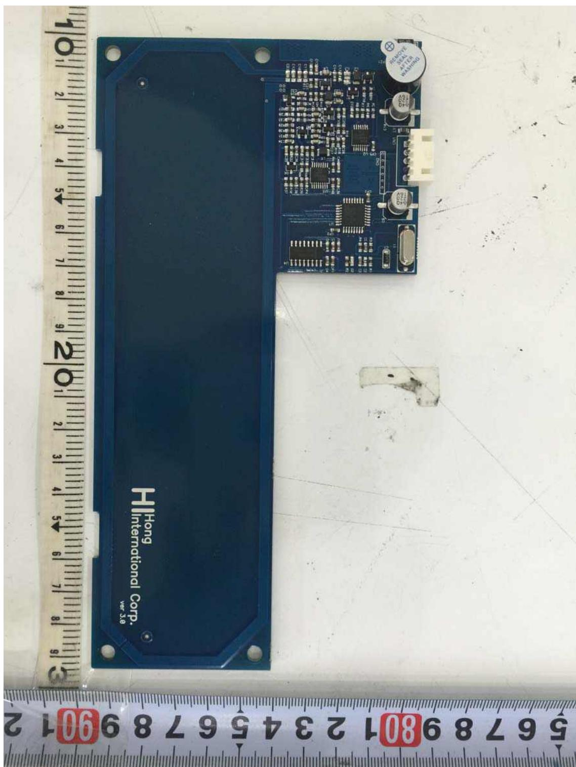
View of RFID PCB(Bottom)
