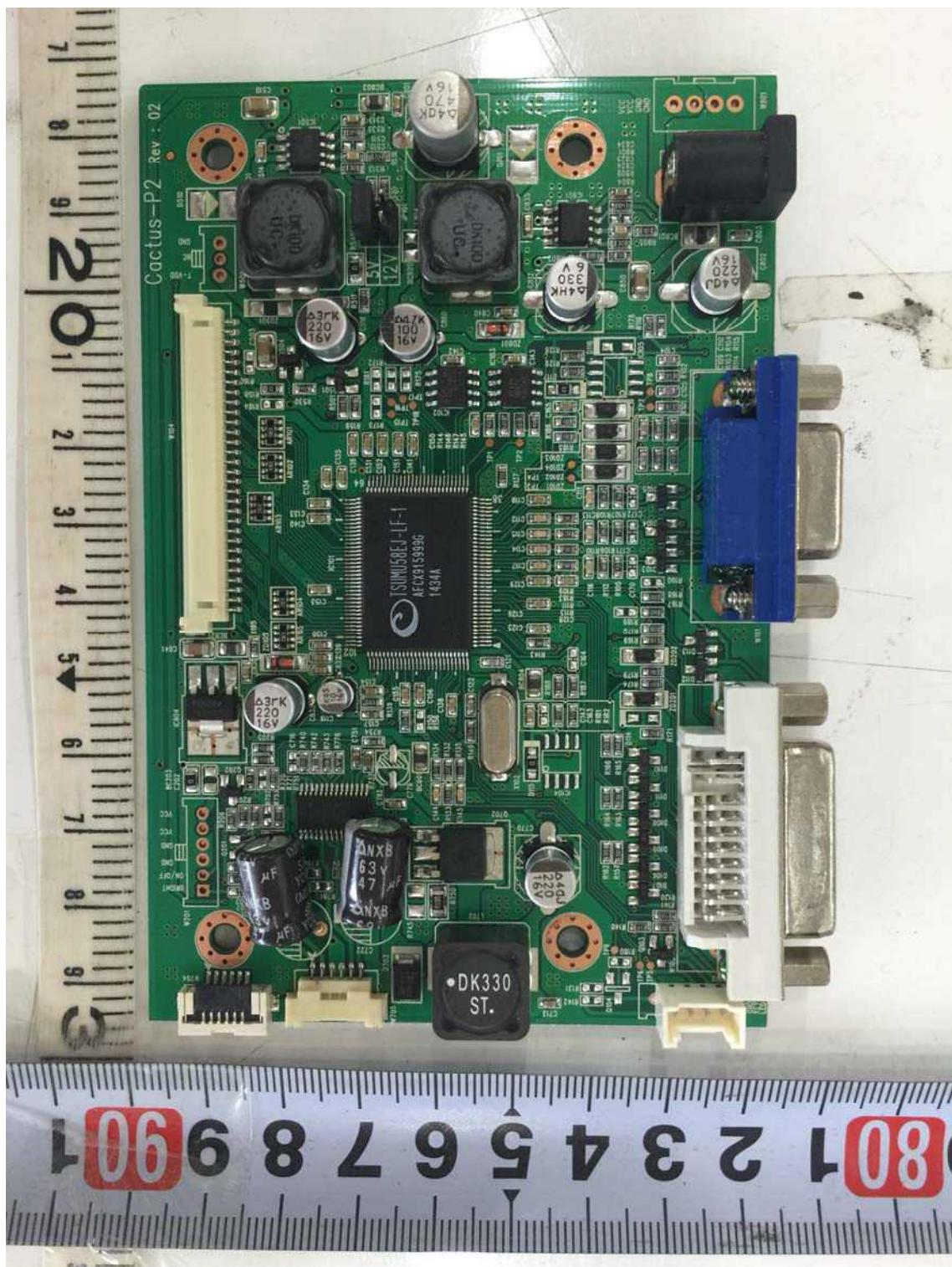
View of Main PCB of Monitor 2(Bottom)
