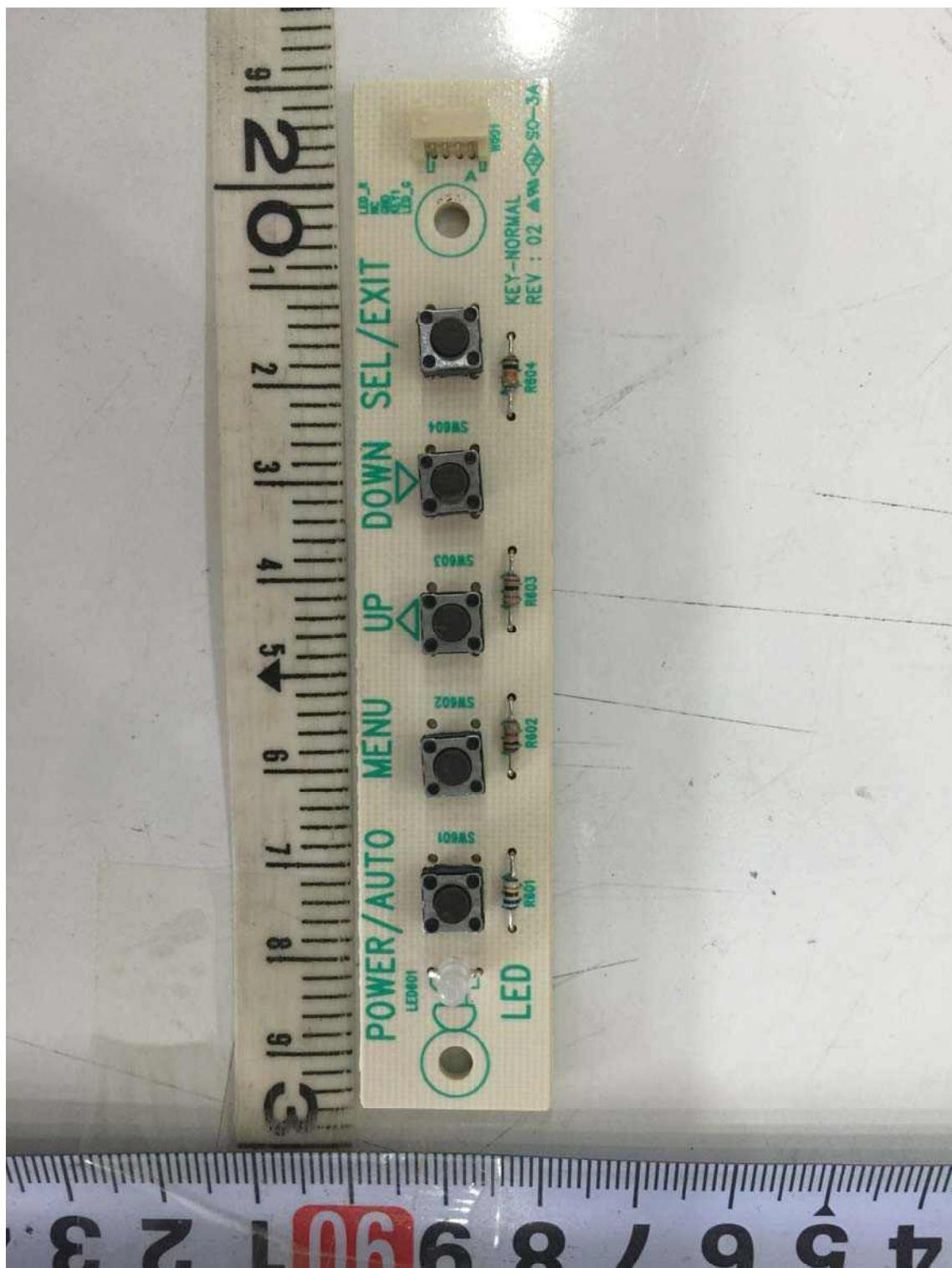
View of Button PCB of Monitor 1(Bottom)
