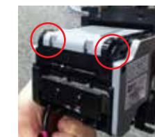
Locking lever on bill acceptor lense
