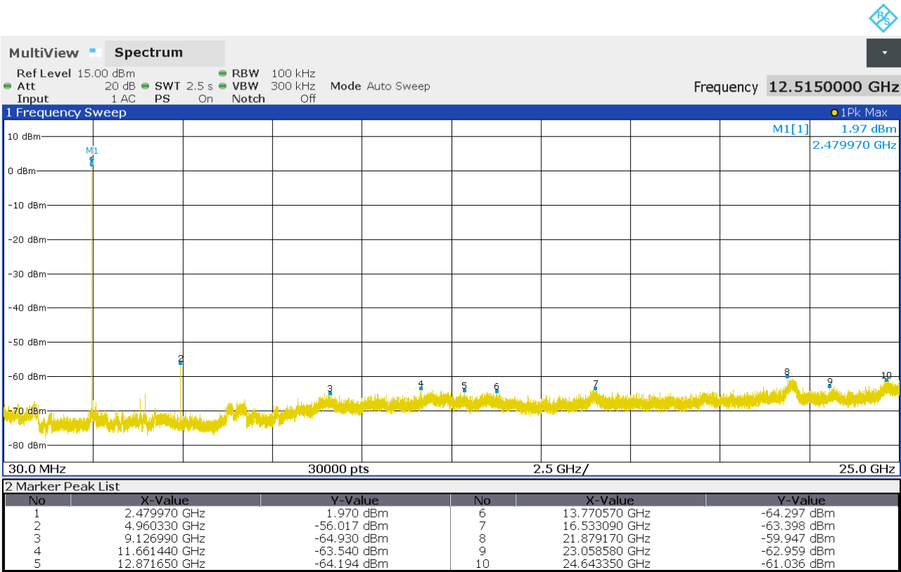
Figure 15 Conducted emissions 30MHz to 25GHz. Operation on channel 2480MHz.
