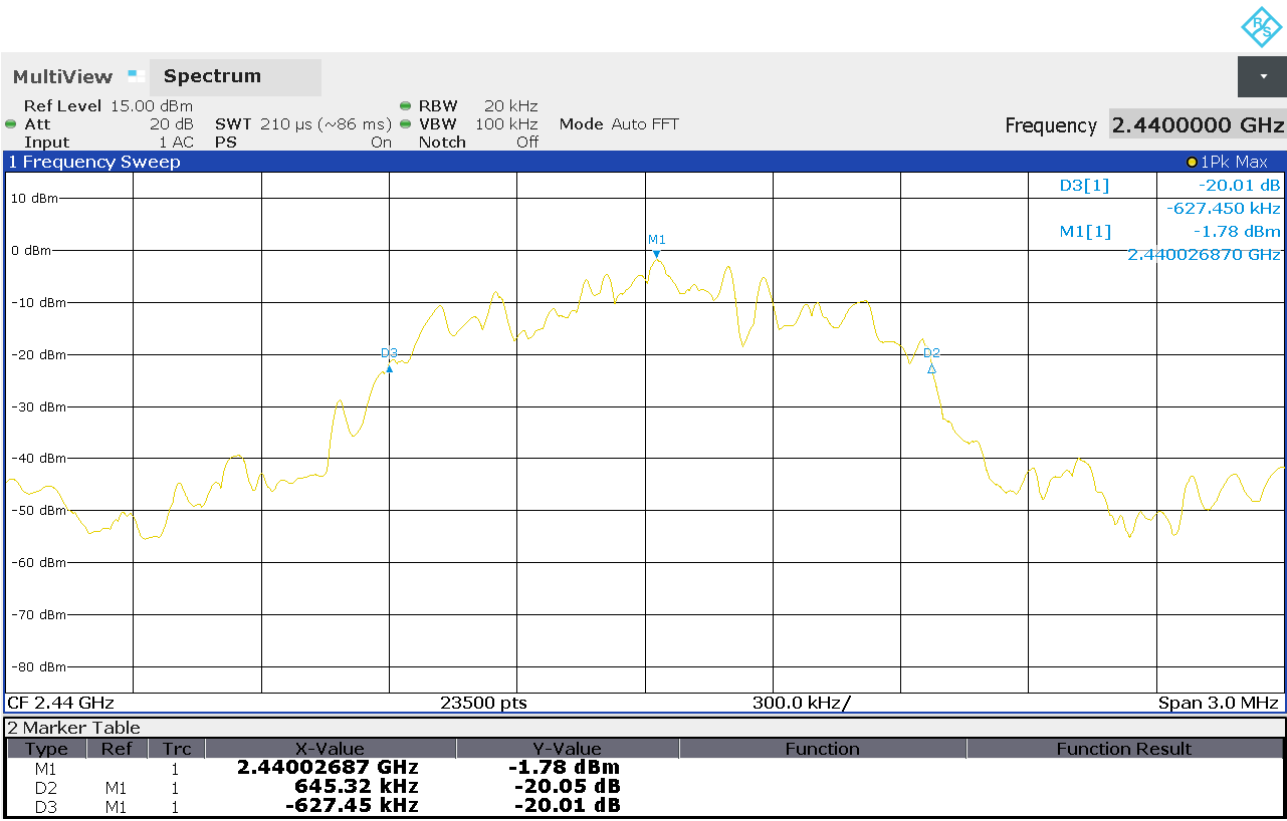
Figure 17 Bandwidth at 20dB Point. Operation on channel 2440MHz
