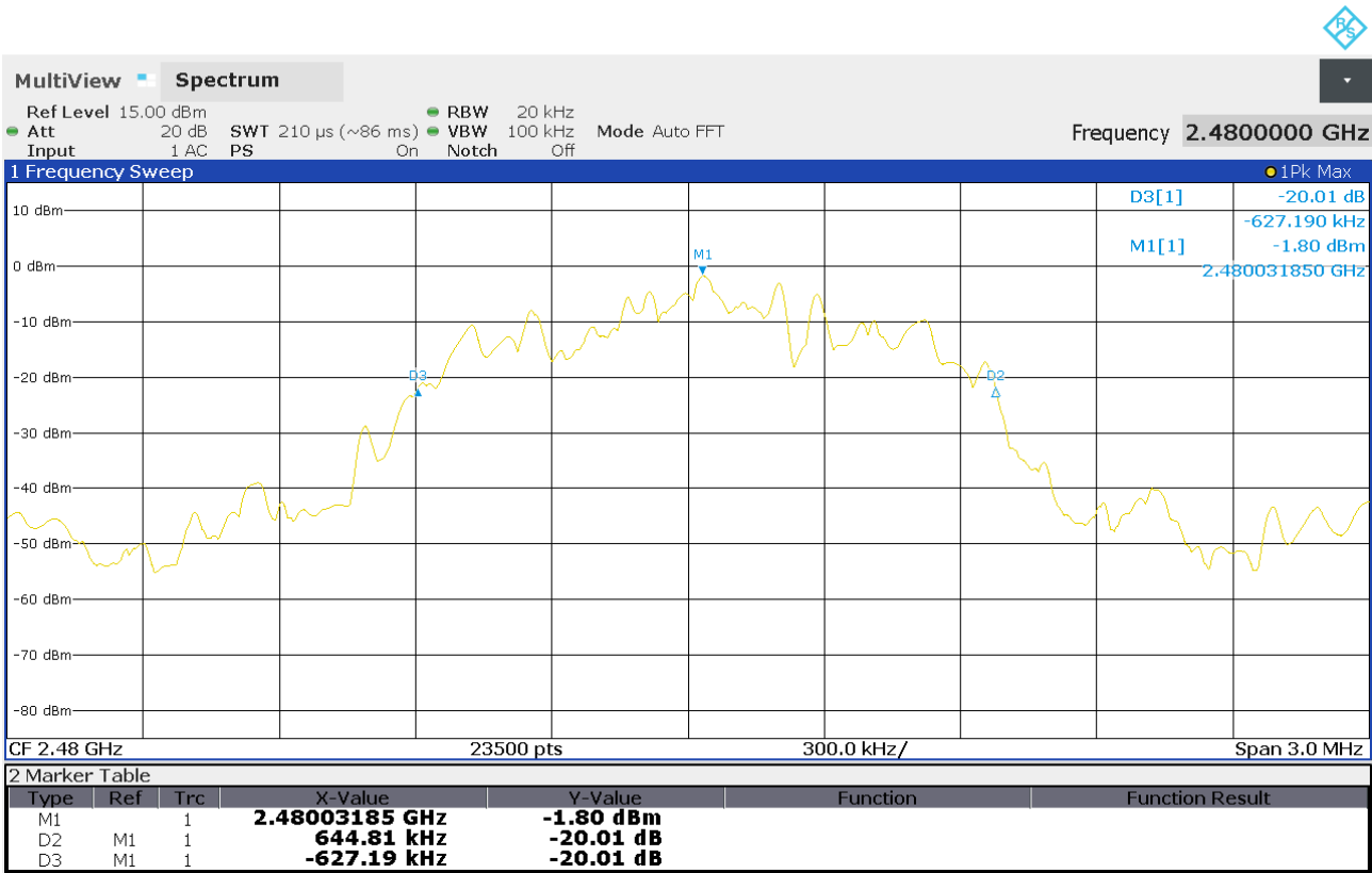
Figure 18 Bandwidth at 20dB Point. Operation on channel 2480MHz
