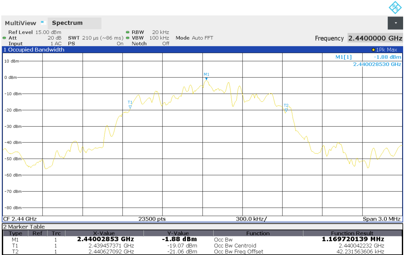
Figure 20 99% Occupied Bandwidth. Operation on channel 2440MHz
