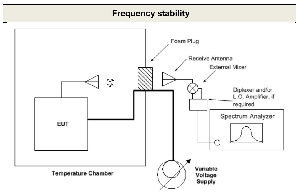
**■ Test Procedure:****ANSI C63.10-2020 – Section 9.5**
