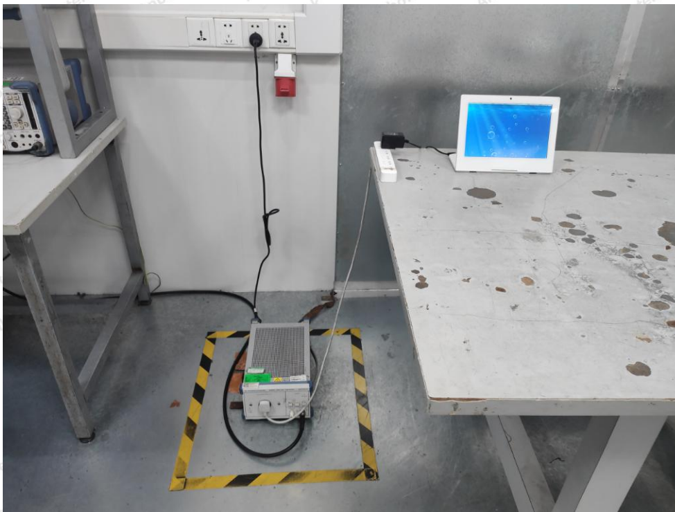
Photo of Power Line Conducted Emission Test
