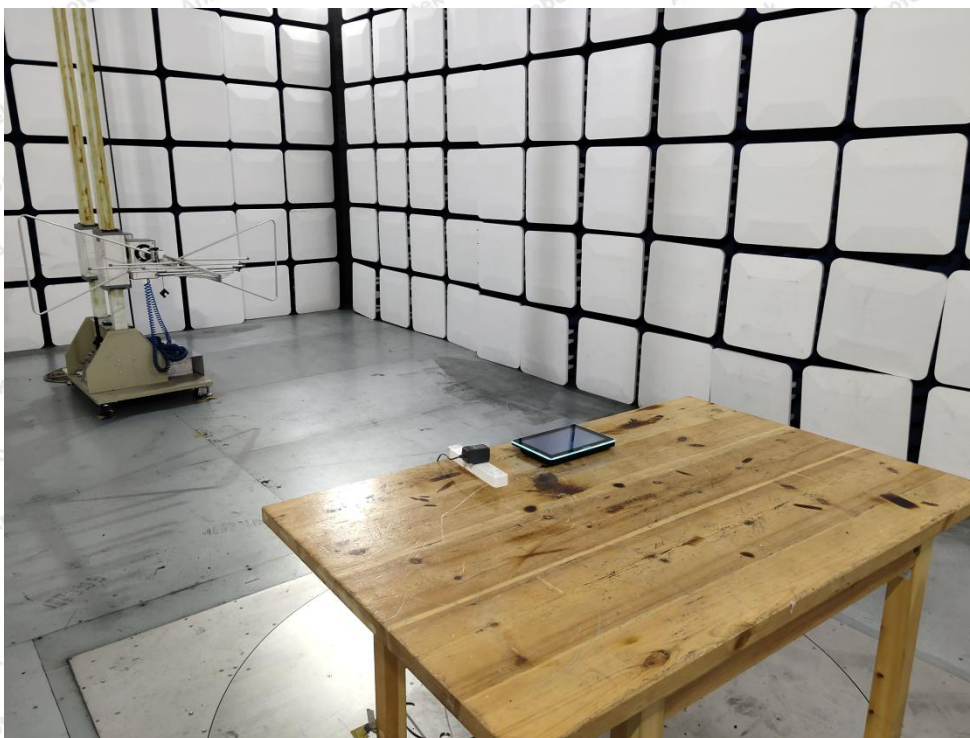
Photo of Radiation Emission Test
