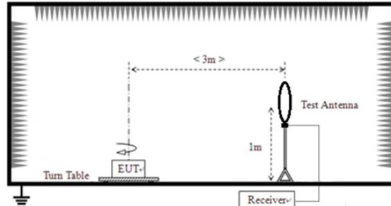
For radiated emissions from 30MHz to 1GHz
