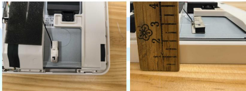
Remark: the distance calculated is the antenna installation location to touch screen, simultaneous transmission not support
