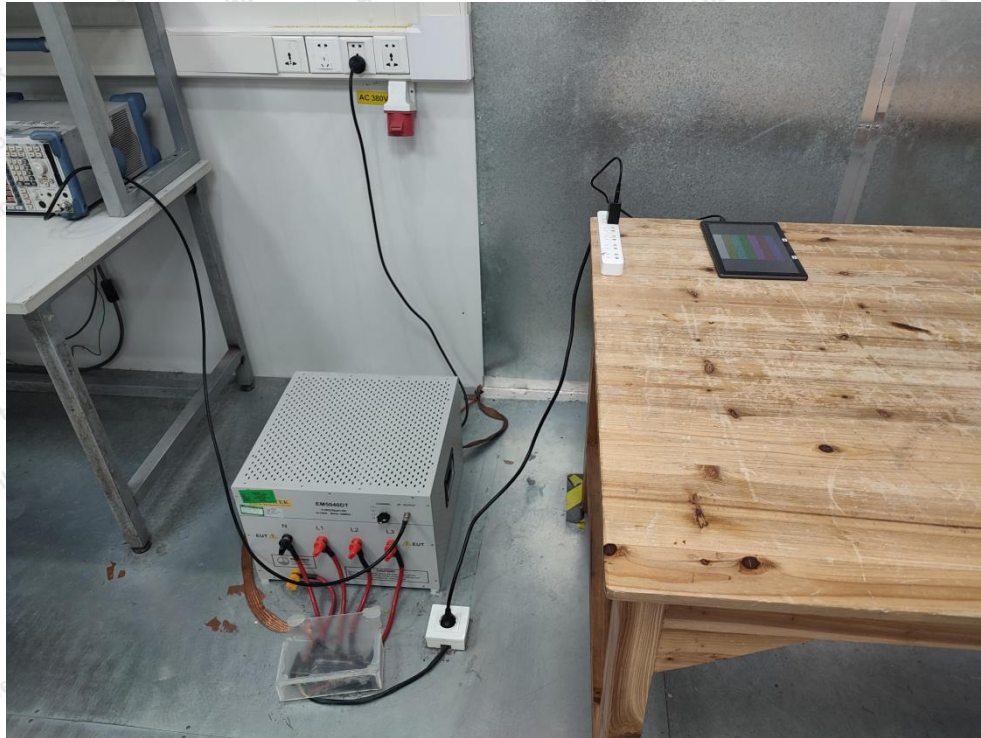
Photo of Conducted Emission Measurement
