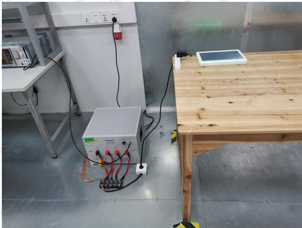
Photo of Power Line Conducted Emission Test
