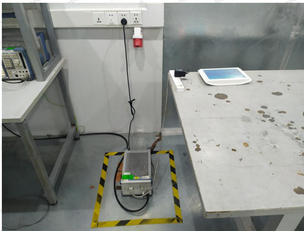
Photo of Power Line Conducted Emission Test
