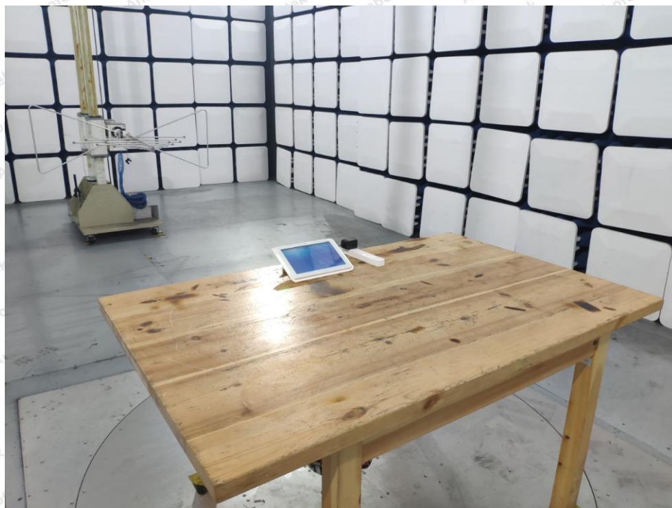
Photo of Radiation Emission Test
