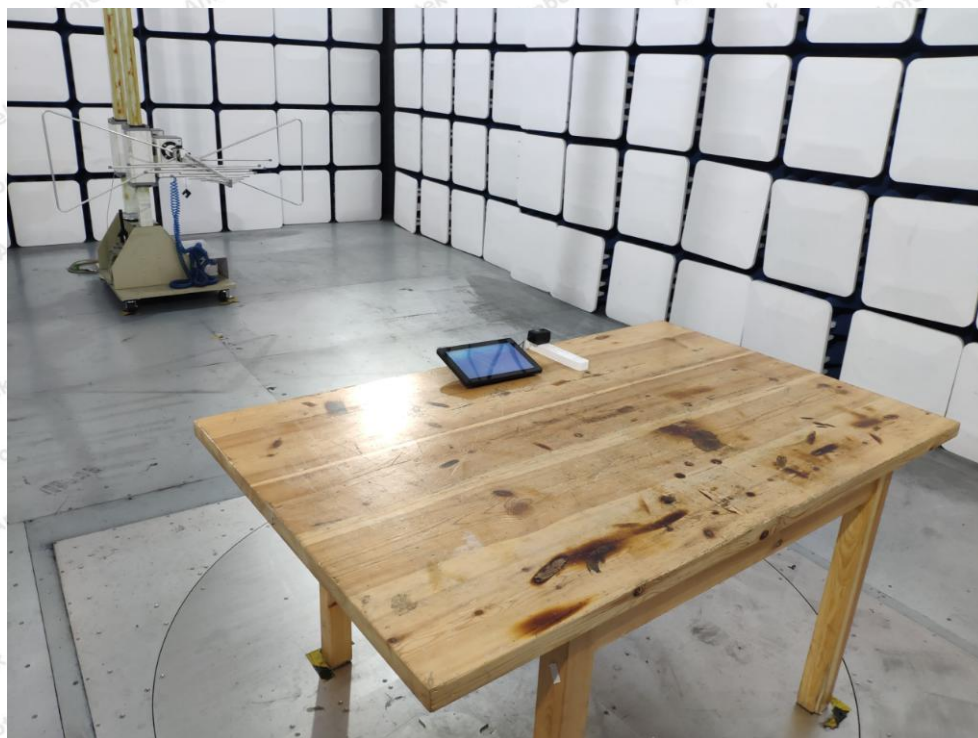
Photo of Radiation Emission Test
