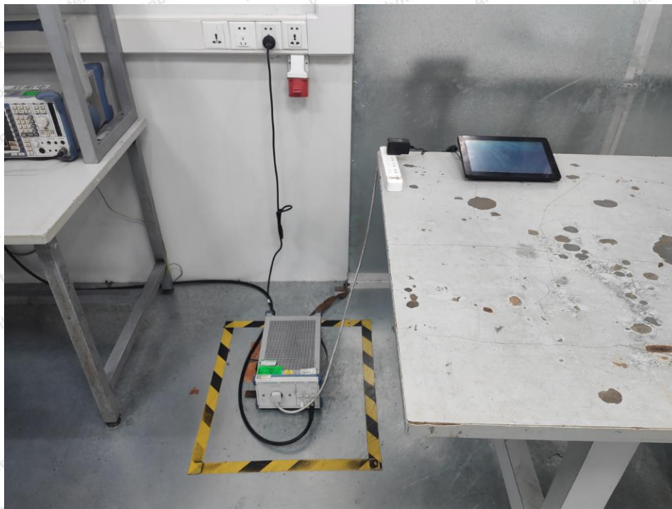
Photo of Power Line Conducted Emission Test
