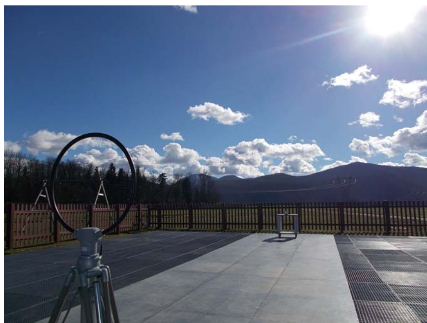
Figure 2: Radiated emission test – OATS measurements
