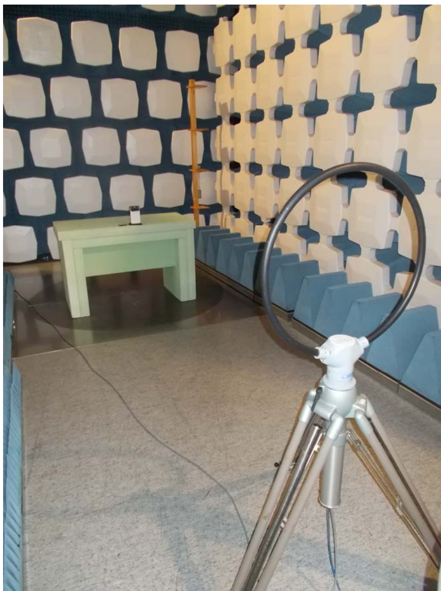
Figure 3: Radiated emission test – below 30 MHz
