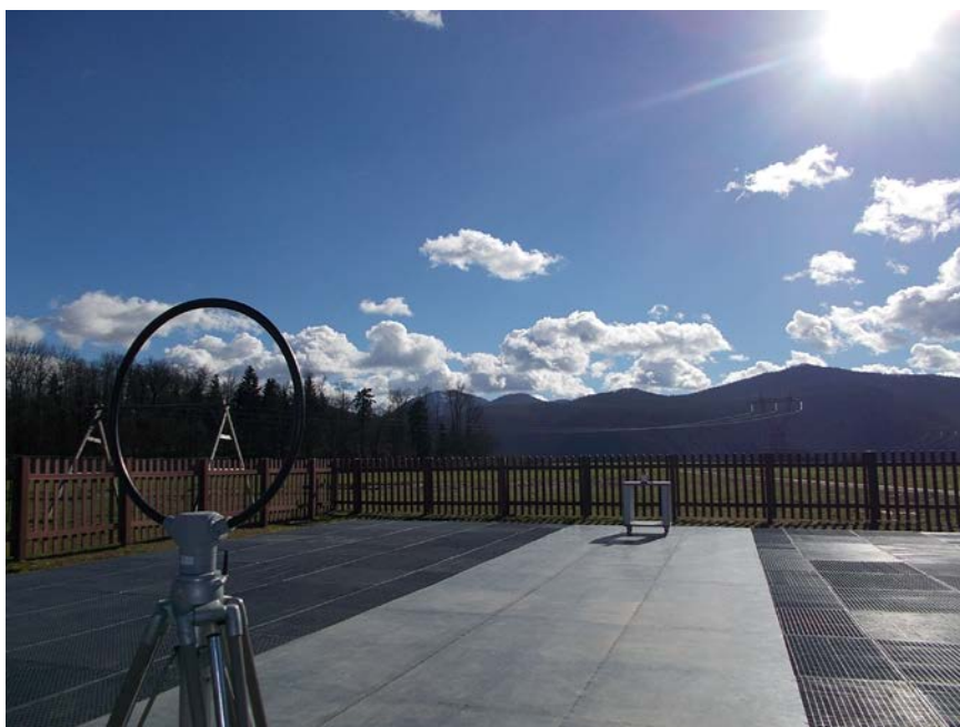
Figure 2: Radiated emission test – OATS measurements
