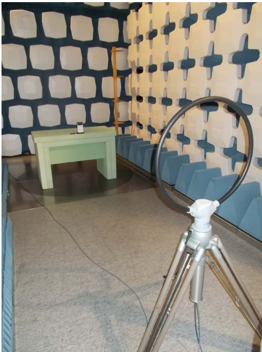
Figure 3: Radiated emission test – below 30 MHz
