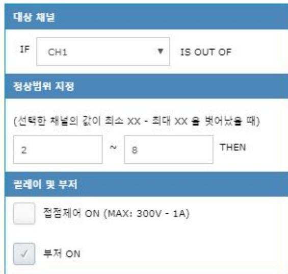
Dry Contact only works when the DC power supply is connected.(However, batteries should be inserted even when connecting to DC power.)Contact control can operate a warning light or fan.
