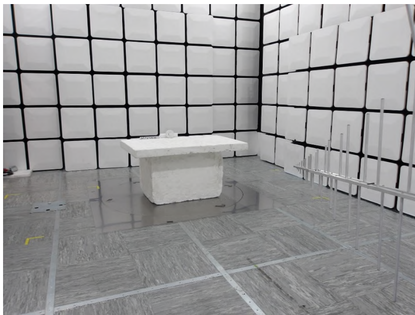
Photo 1.5-1 – Radiated Spurious Emission 30M-1G Test Setup Photo [Front View]
