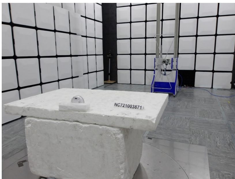
Photo 1.5-2 – Radiated Spurious Emission 30M-1G Test Setup Photo [Back View]
