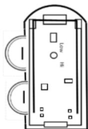
Slide the batteries out from under the circuit board and insert new batteries observing polarity
