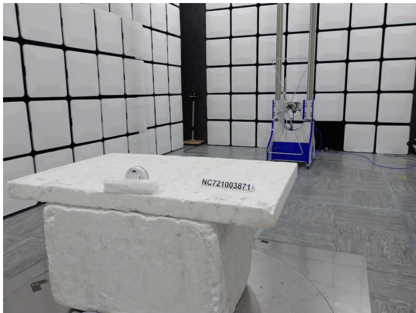
Photo 1.4-2 – Radiated Fundamental Field Strength Test Setup Photo [Back View]
