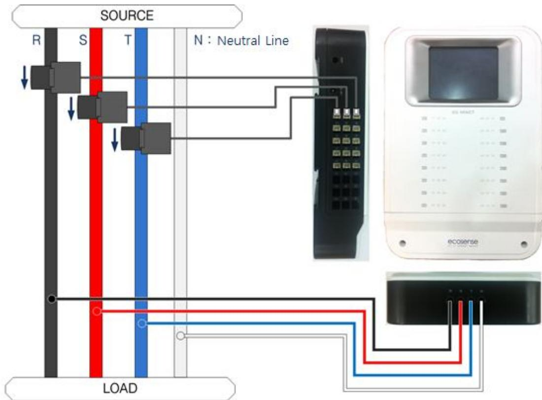
\* It is possible to measure 16 channel with 3 phase 4 wire connection.
