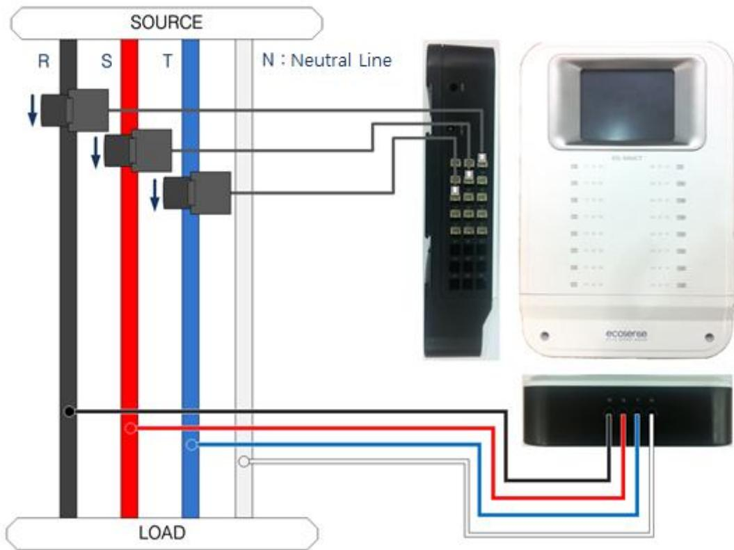
\* It is possible to measure 48 channel with single phase 2 wire connection.
