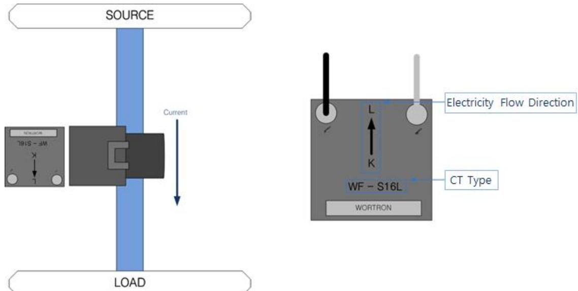
Electricity Flow Direction : K = SOURCE, L = LOAD
