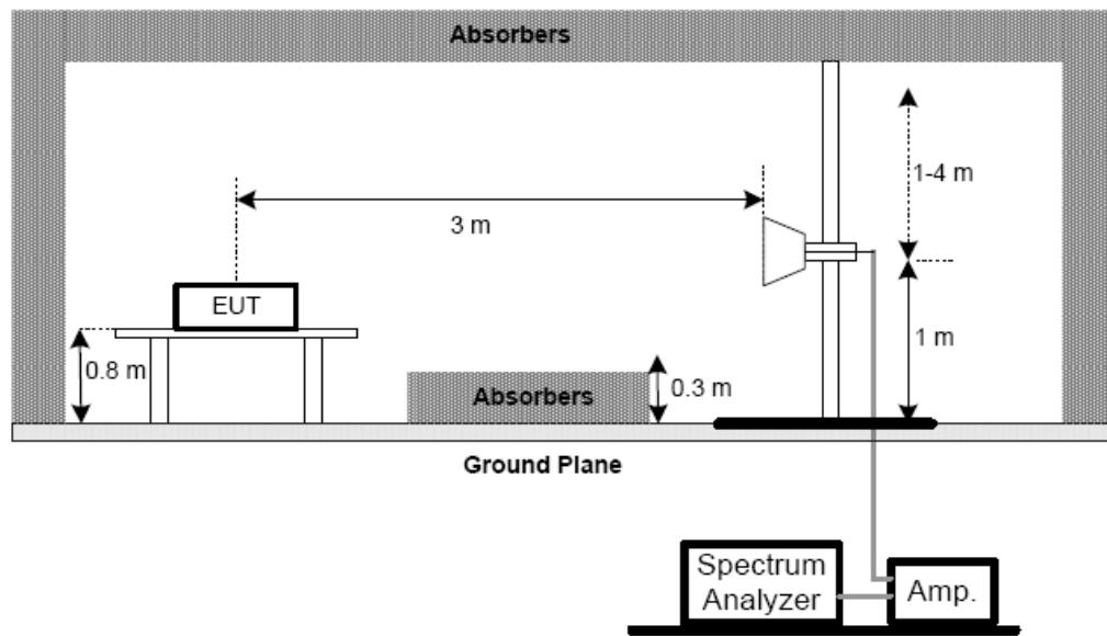
(C) For radiated emissions below 30MHz
