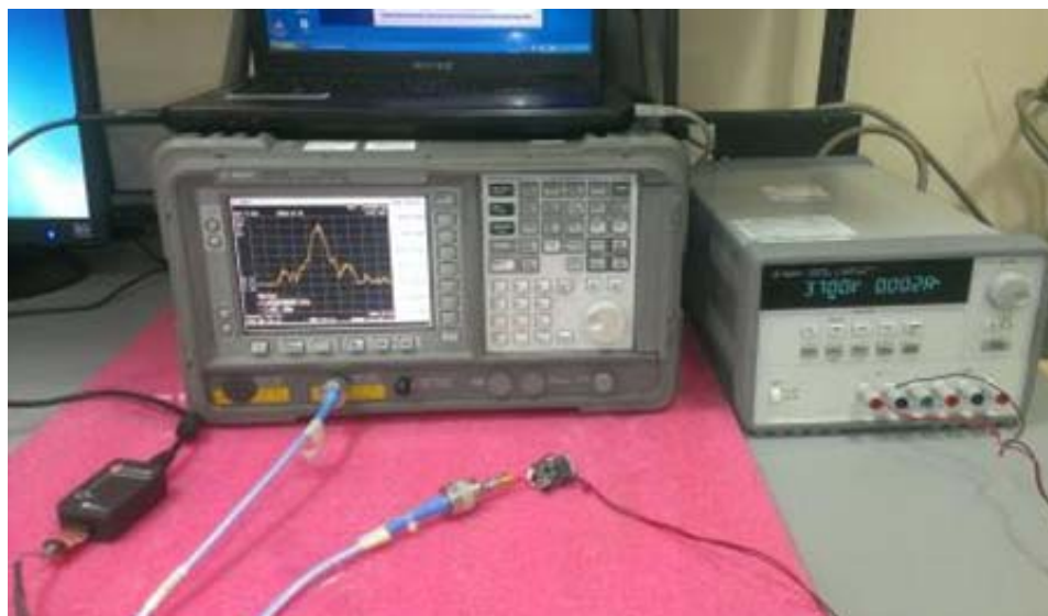
Figure 8: Test setup for Conducted Measurements
