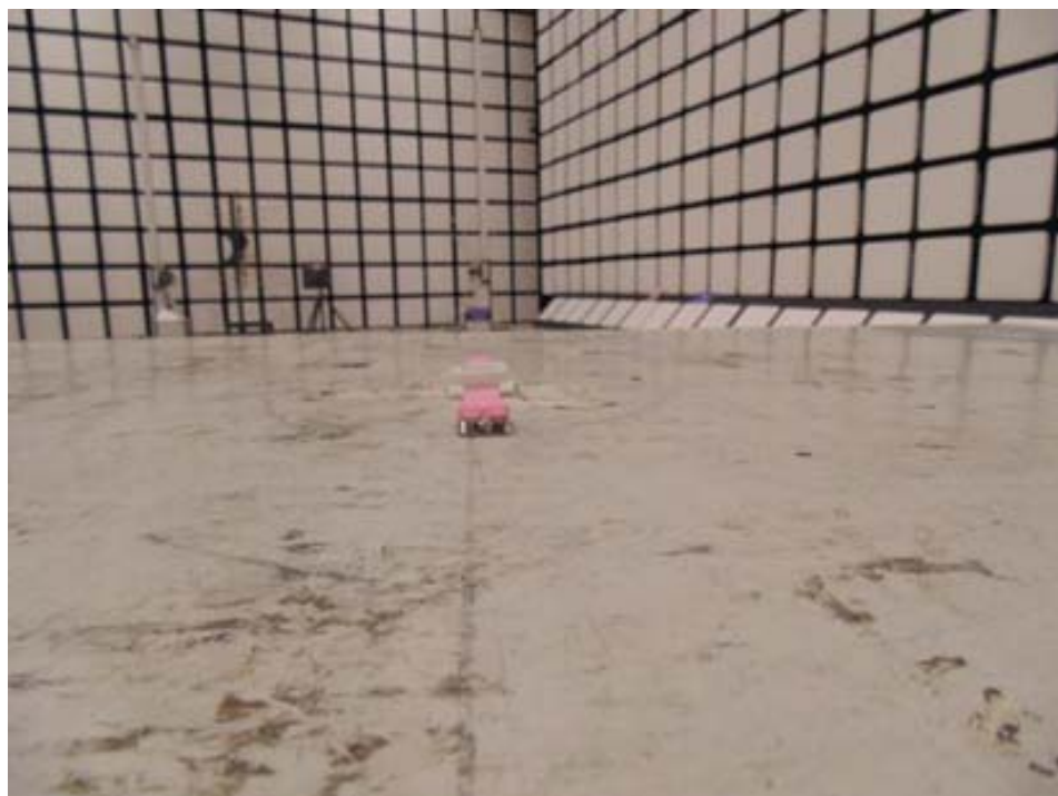
Figure 3: Test setup for Radiated Emission 30MHz to 1GHz - Vertical Polarization
