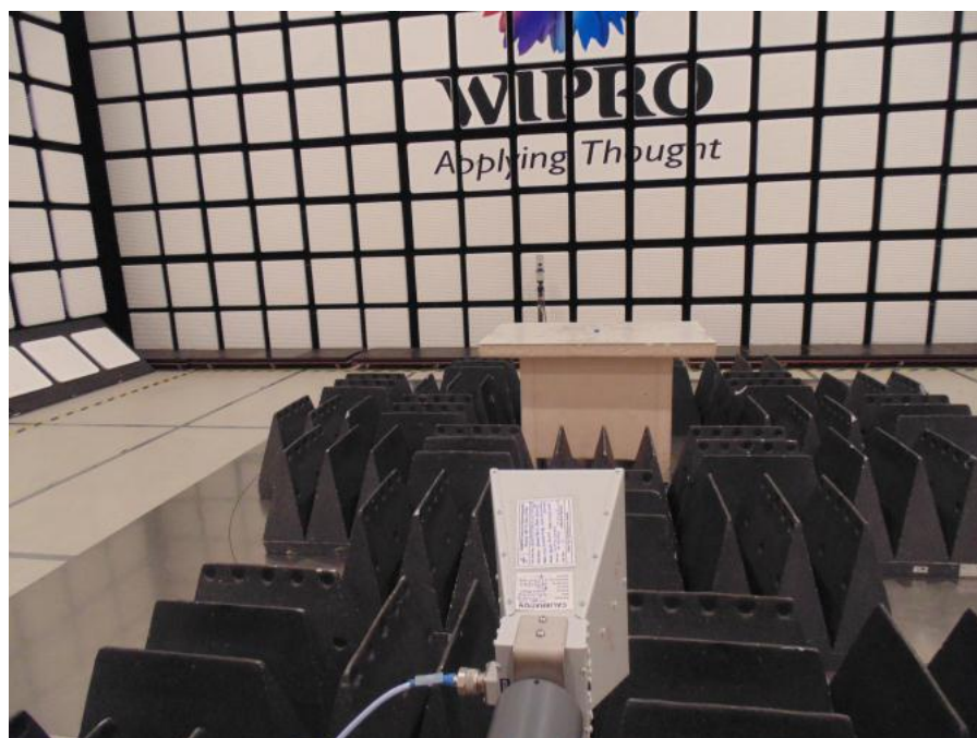
Figure 4: Test setup for Radiated Emission from 1GHz to 18GHz – Horizontal Polarization
