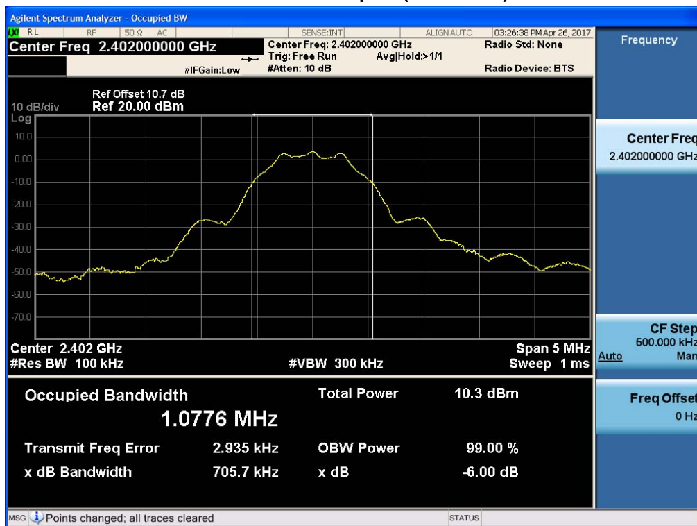
6 dB Bandwidth plot (Low-CH 0)
