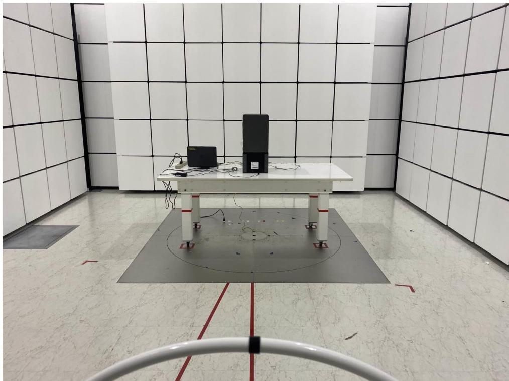
**Radiated emissions test photos****30 MHz to 1 GHz**
