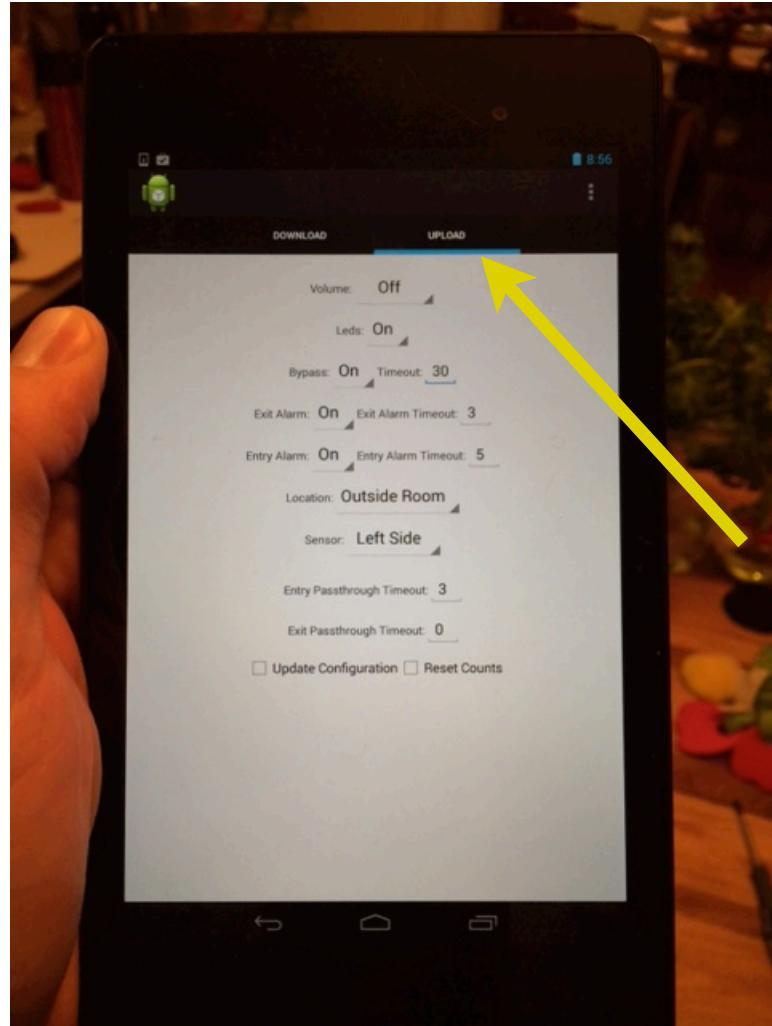
10. Change any of the desired values. Hold the tablet back up to the Sanicheck and wait for the beep followed by UI zoom. The message will once again appear "Touch to Beam". This time, **TOUCH THE SCREEN to beam the new configuration to the Sanicheck as in the next photo.**
