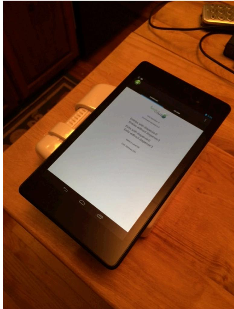
8. Pull the tablet away from the Sanicheck unit and wait for the beep to indicate disconnection. Data download is now complete.
