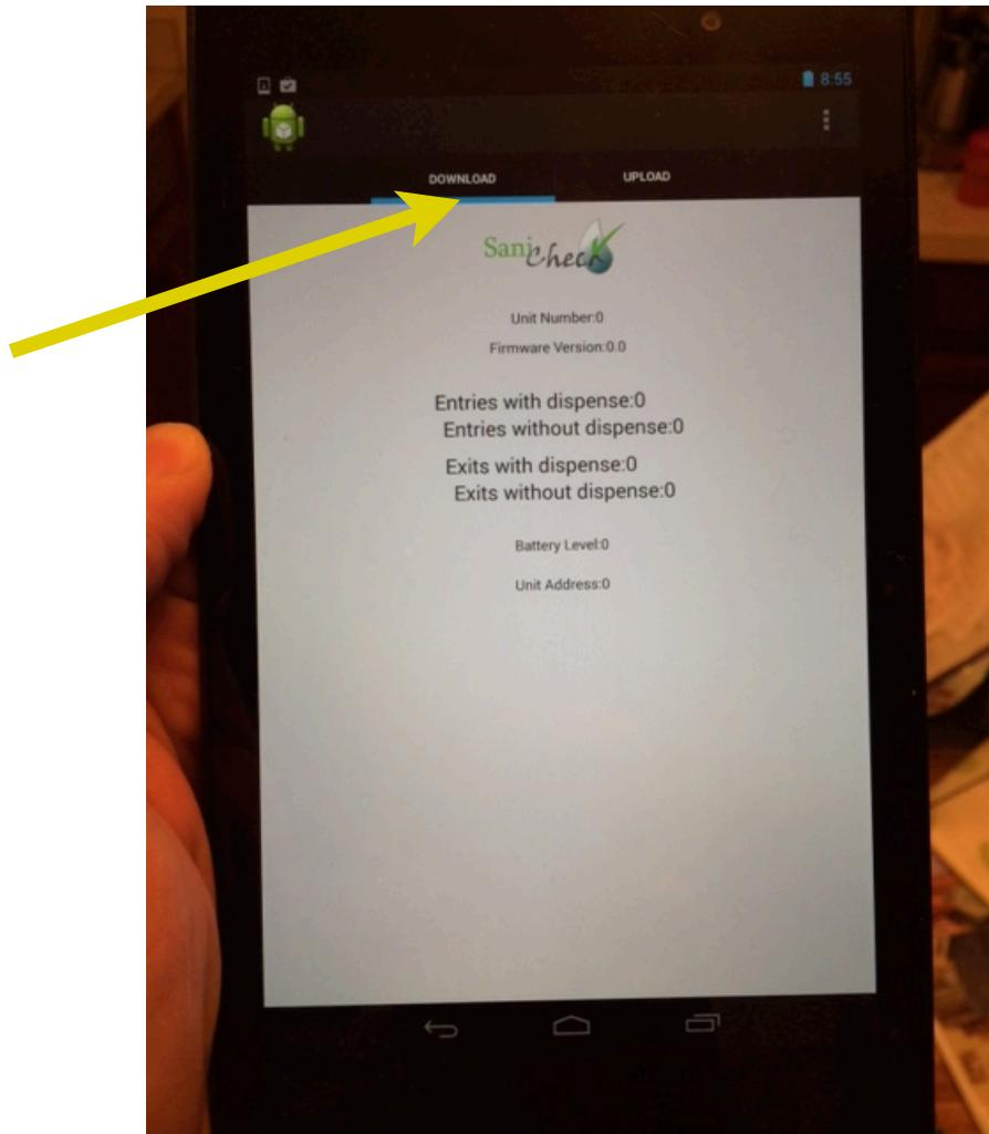
7. Hold the back of the table up against the front of the Sanicheck unit as in the next photo. The Sanicheck unit will beep. The Tablet UI will zoom out slightly and a message will be displayed "Touch To Beam". **DO NOT TOUCH THE SCREEN at this time.** Wait approximately 5 seconds, and the data will automatically transfer.
