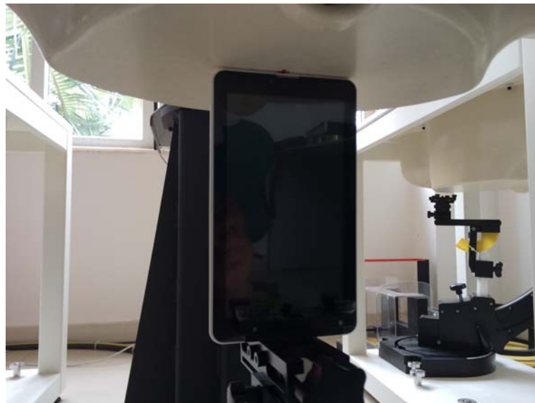
0mm Body-worn Top Side Setup Photo
