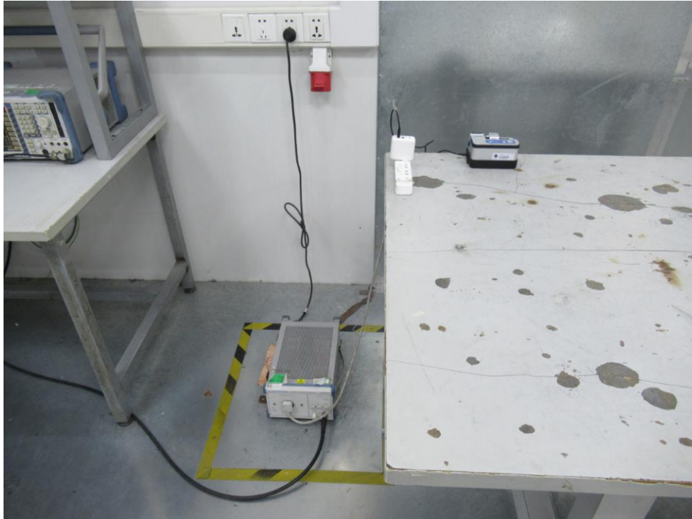
Photo of Power Line Conducted Emission Test
