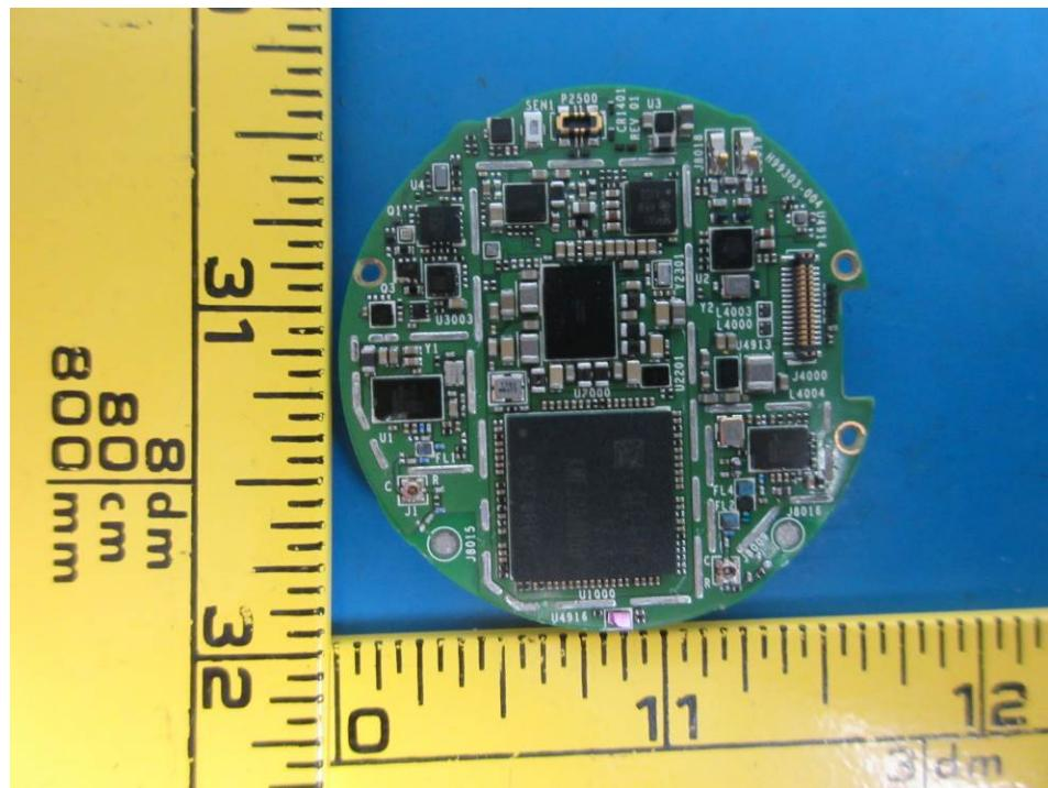
**11.9 EUT Main Board Bottom View w/ Battery**
