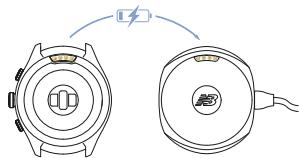
Connect the RunIQ charger to a 5V, 1A USB charging port and place the RunIQ on the charger with the contacts aligned.
